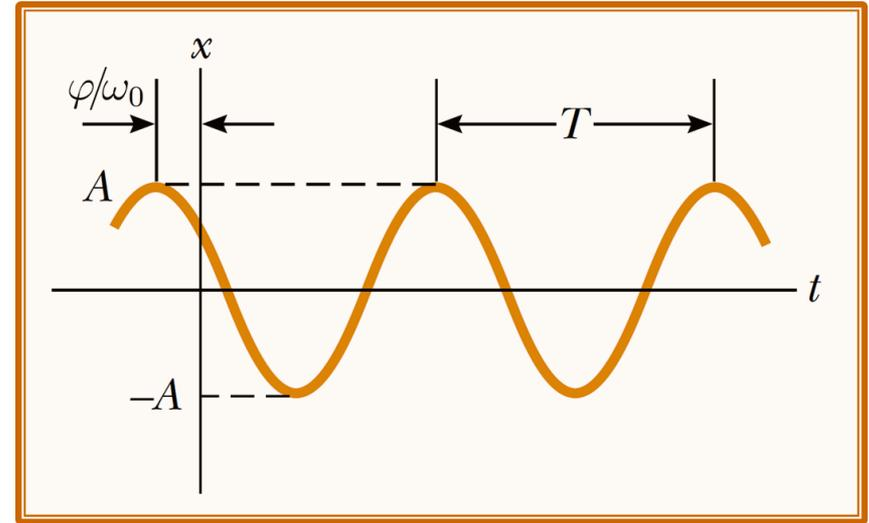
$$\left. \begin{cases} \textcircled{1} \Rightarrow A \cos \varphi = x_0 \Rightarrow A^2 \cos^2 \varphi = x_0^2 \\ \textcircled{2} \Rightarrow A \sin \varphi = -\frac{v_0}{\omega_0} \Rightarrow A^2 \sin^2 \varphi = \frac{v_0^2}{\omega_0^2} \end{cases} \right\} A^2 = x_0^2 + \frac{v_0^2}{\omega_0^2} \Rightarrow A = \sqrt{\frac{v_0^2 + \omega_0^2 x_0^2}{\omega_0^2}}$$
