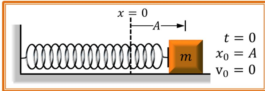
$$\ddot{x} + \omega_0^2 x = 0 \quad \omega_0 = \sqrt{\frac{k}{m}}$$
