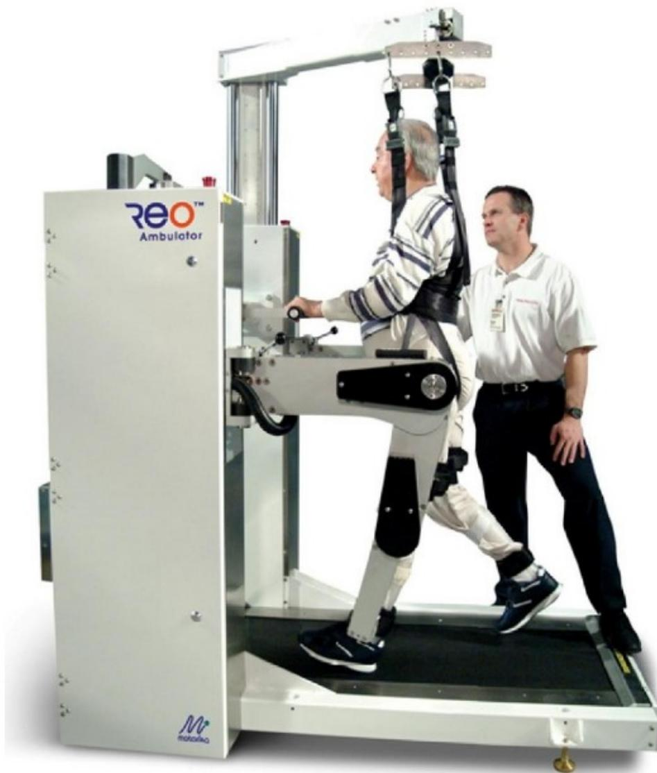
ReoAmbulator robotic system (picture courtesy of Motorika Ltd.).
