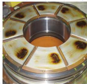
Overheating, Oil Additives Plated Out
