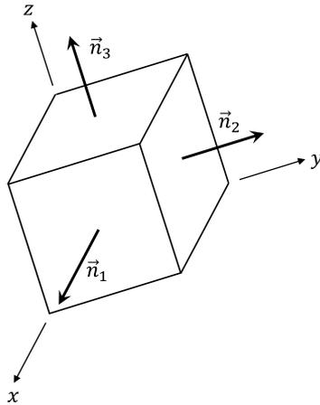
$$[T] = \begin{bmatrix} \sigma_x & 0 & 0 \\ 0 & \sigma_y & 0 \\ 0 & 0 & \sigma_z \end{bmatrix} = \begin{bmatrix} \sigma_1 & 0 & 0 \\ 0 & \sigma_2 & 0 \\ 0 & 0 & \sigma_3 \end{bmatrix}$$
