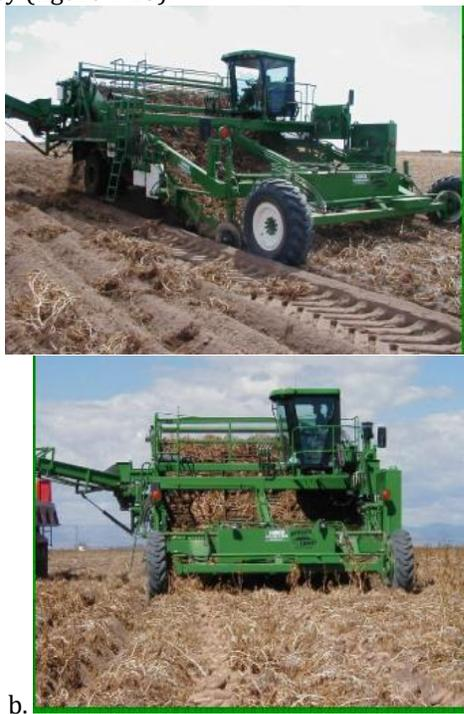
Figure 4.15. Straight thru potato combine harvester under operation (a and b)
