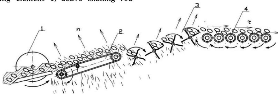
Figure 4.18. Root crop and potato cleaning system [40]
