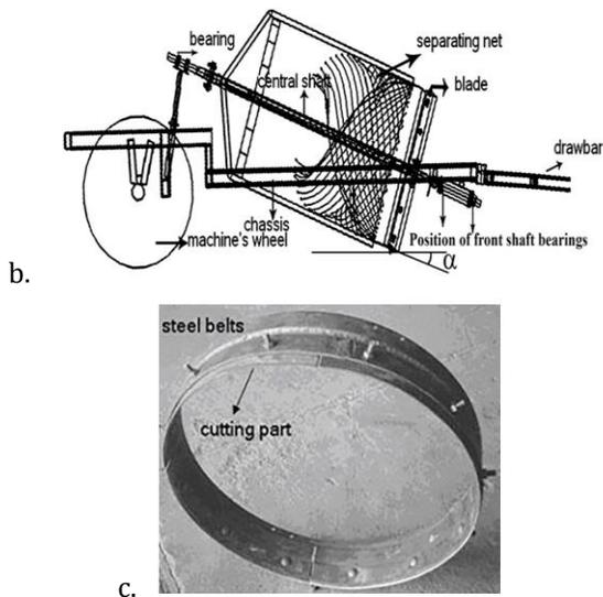
Figure 4.13. Spinner potato harvester (a), rotary potato digger (b), and rotary potato digger blades (c)
