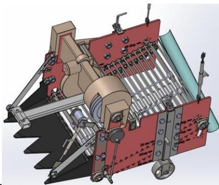
Figure 4.8. Single axle tractor operated potato digger elevator (a), and an isometric view of a machine (b)
