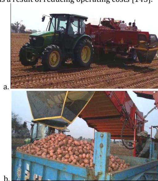
Figure 4.14. The tractor was drawn potato combine harvester (a) and potato combine loading system (b)
