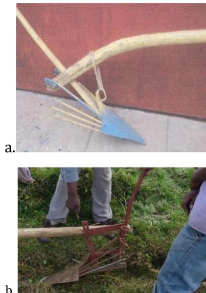
Figure 4.7. Melkassa digger (a) and *Selam* potato lifter (b)
