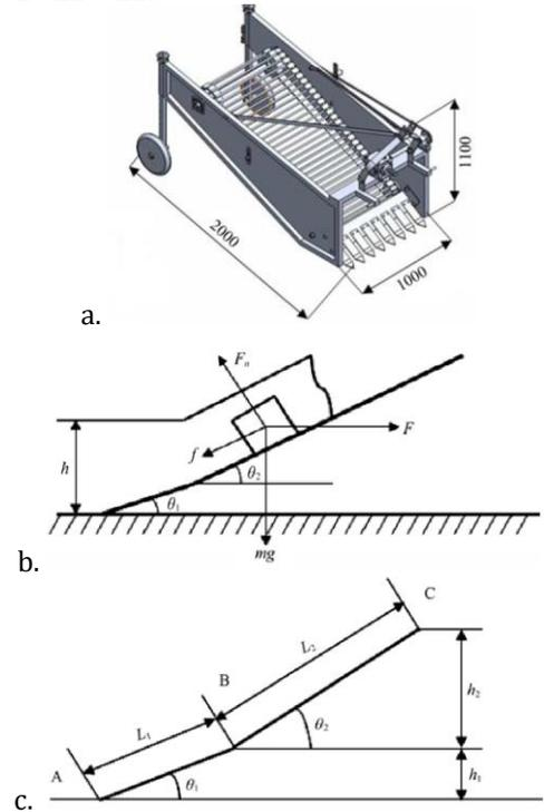
Figure 4.2. Structure of the digger blade (a), force diagram of the excavating shovel (b), and calculation length of the excavation mechanism (c) [90]
