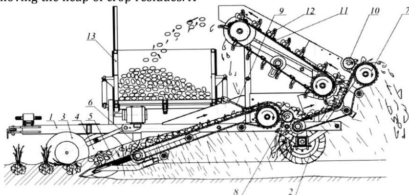
Figure 4.19. Design and process flow sheet of a potato harvesting machine (14)
