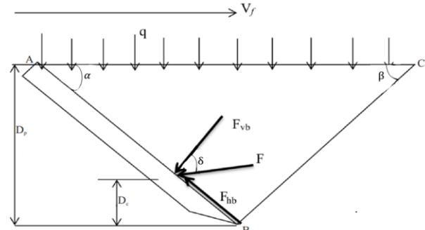
Figure 4.1. Diagram of the soil reactions acting on a blade [23]
