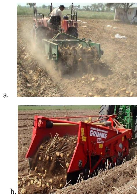
Figure 4.12. Different types of potato digger elevator (a, b, and c)
