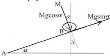
Figure 4.3. Force analysis of digging shovel (Tarek et al., 2016)
