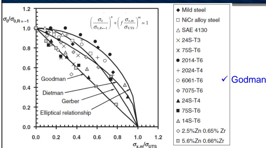
2.6 Accuracy of the considered criteria in predicting the mean stress effect under uniaxial fatigue loading (data from Frost *et al.*, 1974).
