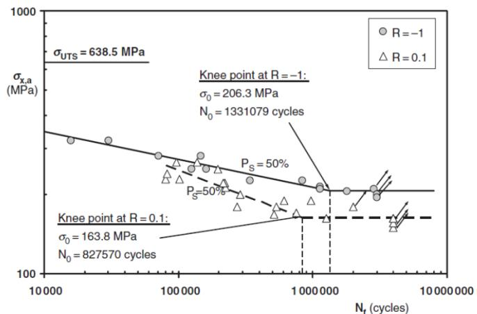
2.5 Fatigue results generated by testing plain flat specimens of En3B under uniaxial loading with a load ratio,  $R$ , equal to both  $-1$  and  $0.1$  (Susmel and Taylor, 2007).
