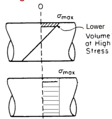
$$S_e(\text{axial}) \approx 0.70S_e(\text{bending})$$
