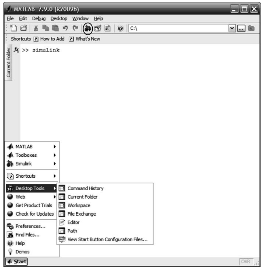
FIGURE C.1 MATLAB Window showing how to access Simulink. The Simulink Library Browser button is shown circled.
