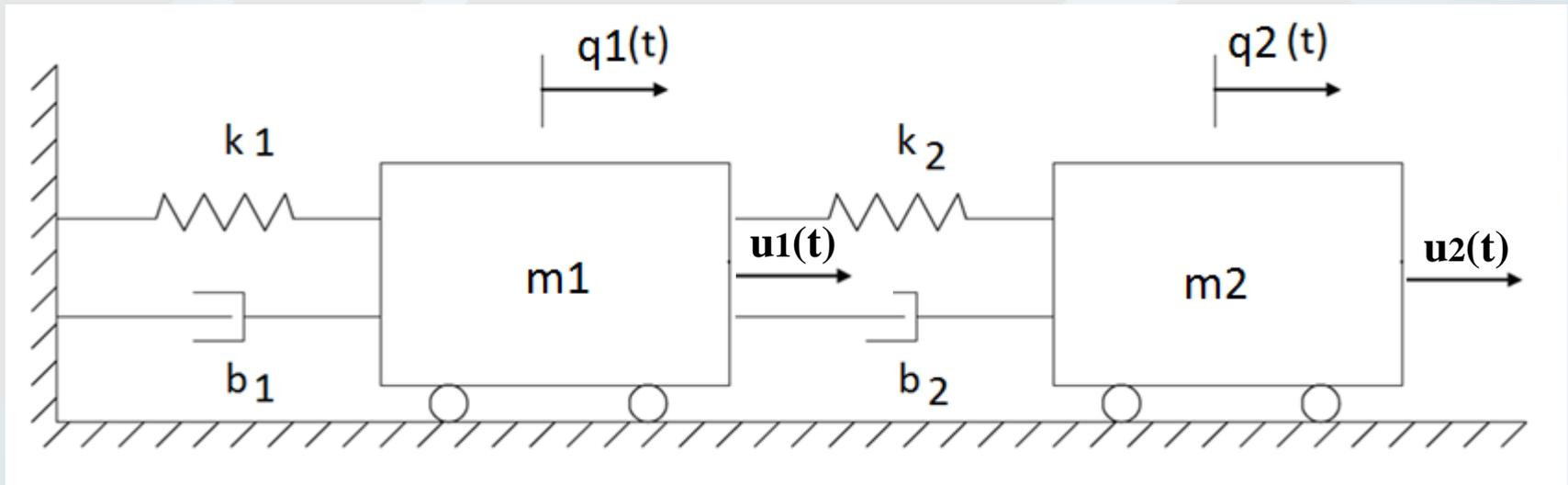
$$\underbrace{\begin{bmatrix} m_1 & 0 \\ 0 & m_2 \end{bmatrix}}_{\mathbf{M}} \begin{bmatrix} \ddot{q}_1 \\ \ddot{q}_2 \end{bmatrix} + \underbrace{\begin{bmatrix} b_1 + b_2 & -b_2 \\ -b_2 & b_2 \end{bmatrix}}_{\mathbf{B}} \begin{bmatrix} \dot{q}_1 \\ \dot{q}_2 \end{bmatrix} + \underbrace{\begin{bmatrix} k_1 + k_2 & -k_2 \\ -k_2 & k_2 \end{bmatrix}}_{\mathbf{K}} \begin{bmatrix} q_1 \\ q_2 \end{bmatrix} = \underbrace{\begin{bmatrix} u_1 \\ u_2 \end{bmatrix}}_{\mathbf{U}}$$
