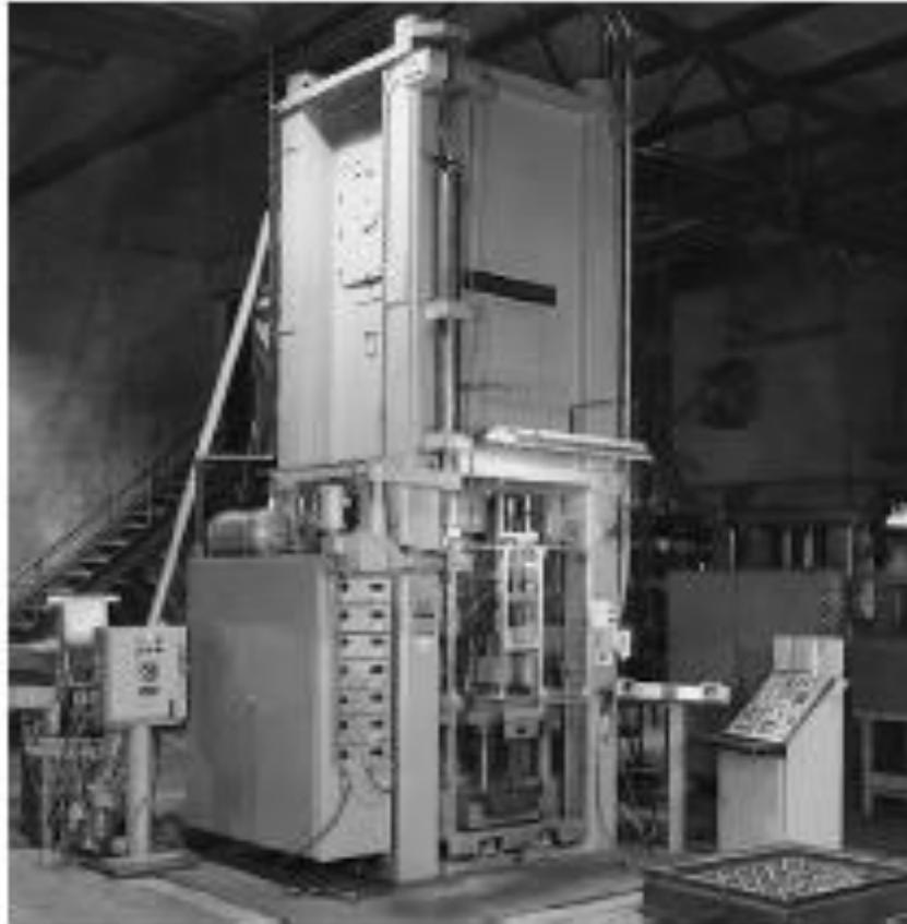
A 7.3 MN (825 ton) mechanical press for compacting metal powder. Source: Courtesy of Cincinnati Incorporated.
