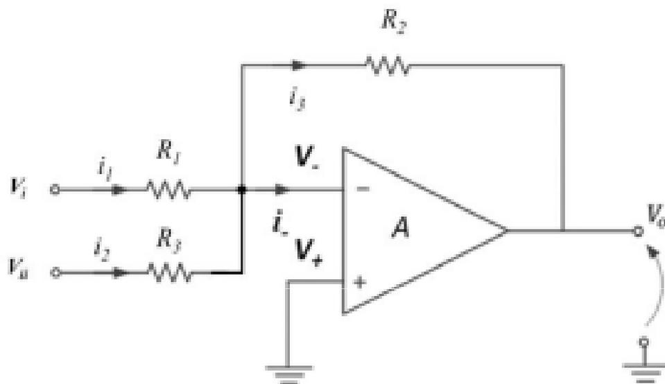
$$V_o = -\frac{R_3}{R_1}V_i - \frac{R_3}{R_2}V_{ii}$$
