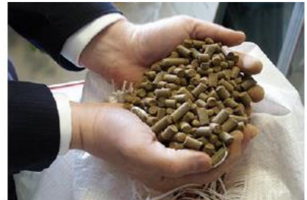
Figure 6. Lignin produced in the demonstration plant at Bäckhammar – filter cake and lignin pellets.
