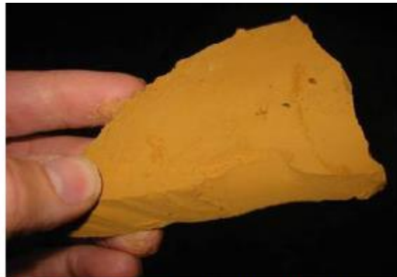
Figure 6. Lignin produced in the demonstration plant at Bäckhammar – filter cake and lignin pellets.
