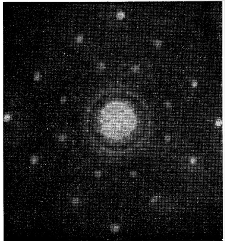
*Left* Laue pattern of x-ray diffraction by a single sodium chloride crystal.
