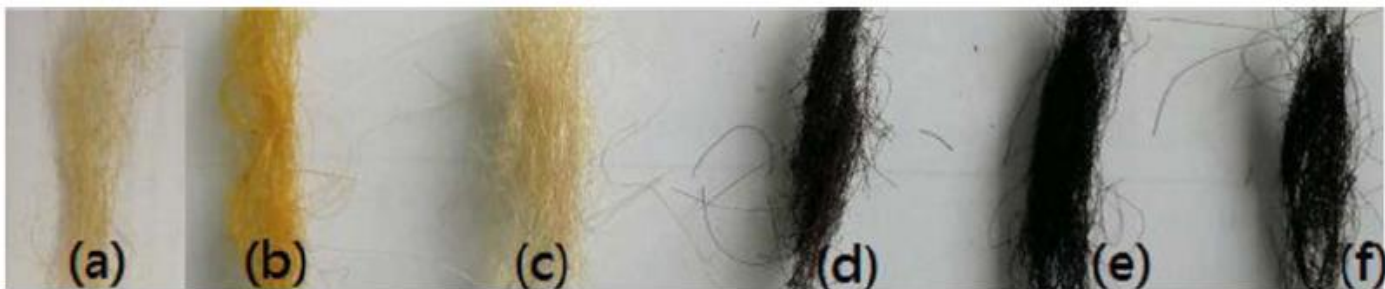
Figure 2. Pictures of different hair samples; (a) bleached hair, (b) laccase treated, (c) dopamine treated, (d) two-step method-I, (e) one-step method, and (f) two-step method-II.
