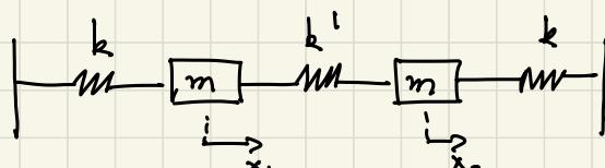
$$T = \begin{bmatrix} m & 0 \\ 0 & m \end{bmatrix} \quad V = \begin{bmatrix} +k + k' & -k' \\ -k' & +k + k' \end{bmatrix} \Rightarrow$$
