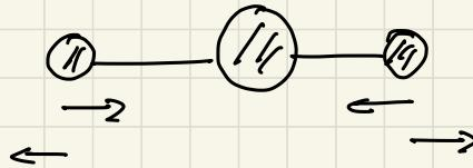
$$\rightarrow \omega_2^2 = k \frac{(2m+m)}{mM} \Rightarrow \begin{pmatrix} \frac{2m}{m} k & k & 0 \\ k & \frac{kM}{m} & k \\ 0 & k & \frac{2mk}{m} \end{pmatrix} \begin{pmatrix} \alpha \\ \beta \\ \gamma \end{pmatrix} = 0$$
