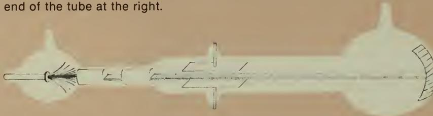
The path of the beam was deflected by an electric field applied between two horizontal plates in the mid-section of the tube; (note that direction of electric field  $\vec{E}$  is upward along plane of page):
