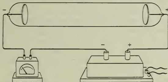
Fig. 2-2 A schematic diagram of a Plücker tube used to study electric currents conducted through gases at low pressures.
