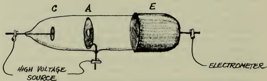
Fig. 2-6 A sketch of another arrangement of anode-cathode placement used by Hertz to show that a cathode ray beam carried no electric charge.
