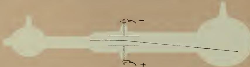
The beam's path was also deflected when there was no electric field but when a magnetic field was set up by means of a pair of current-carrying wire coils placed around the midsection of the tube; (the direction of the magnetic field  $\vec{B}$  is into the plane of the page):
