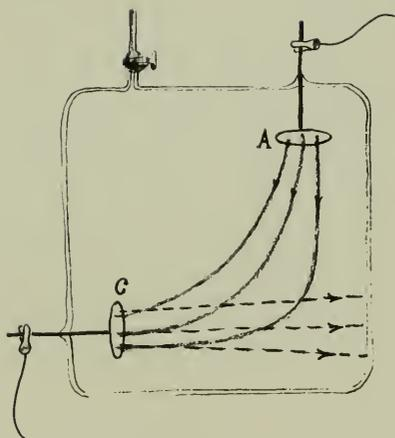
Fig. 2-5 A sketch showing an arrangement of the cathode-anode terminals for an experiment of the type conducted by Hertz to demonstrate the electromagnetic characteristics of cathode rays.
