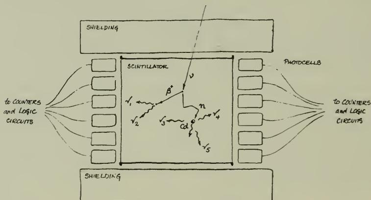
Fig. 4-5 Schematic example of neutrino reaction in a scintillation tank.
