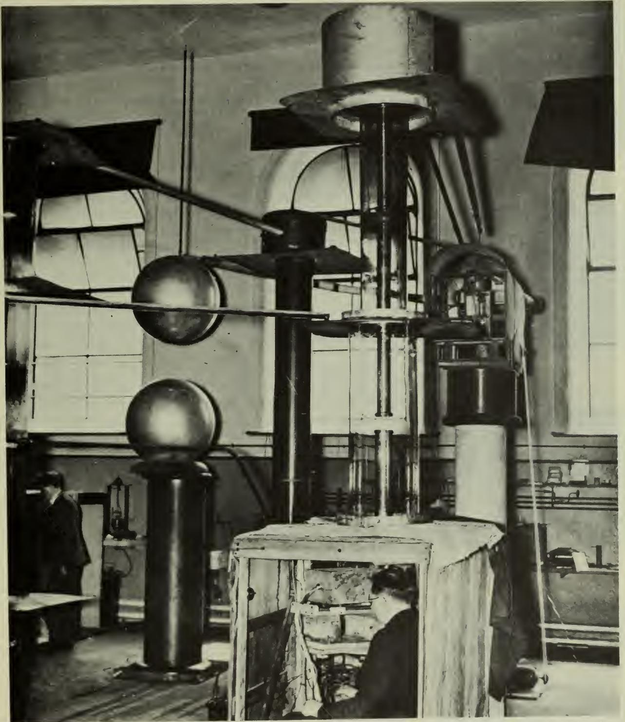
Fig. 4-9 The first successful particle accelerator constructed in 1929 by Cockcroft and Walton at the Cavendish Laboratory.
