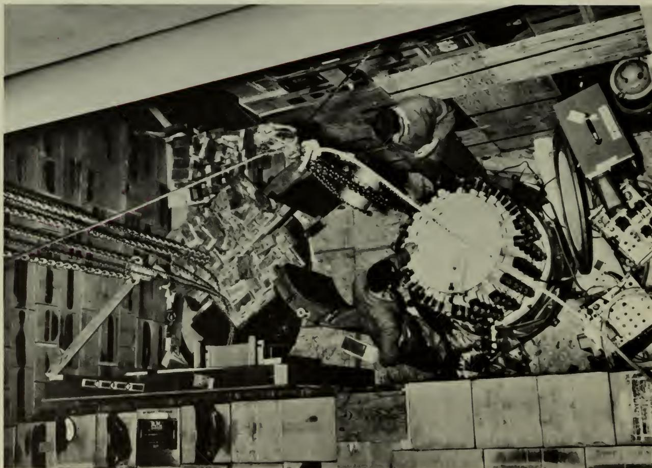
Scintillation counter detector used by Reines and Cowan in their first neutrino experiment at Hanford, Washington, in 1953. The counter, which weighed ten tons, is the cylindrical object at the bottom of the pit.
