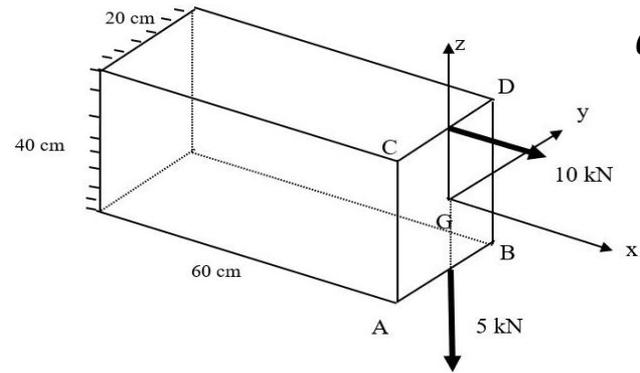
$$a) N = 10kN; |V_z|=5kN; |V_y|=0; M_y = 500 kNm; M_z = 0; T = 0;$$
