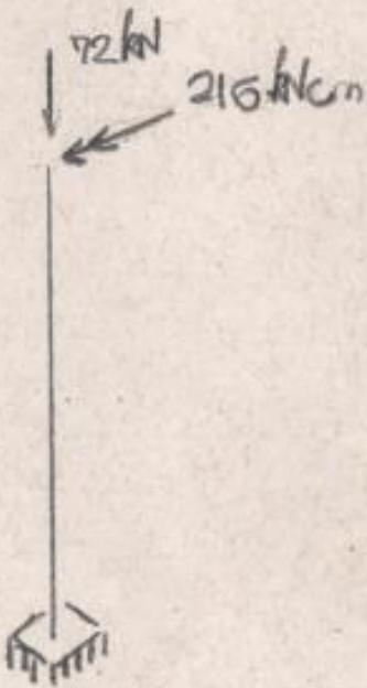
b)  $\sigma = \frac{-72}{72} - \frac{216}{216} z = -1 - z \text{ (em } \text{ kN/cm}^2\text{)}$
