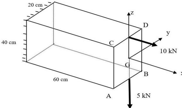
a)  $N = 10 \text{ kN}; |V_z| = 5 \text{ kN}; |V_y| = 0; M_y = 500 \text{ kNm}; M_z = 0; T = 0;$
