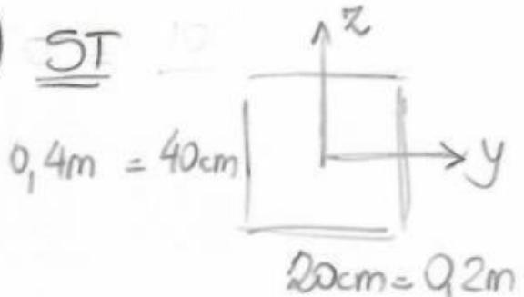
$$A = 0,08 \text{ m}^2 \quad I_y = \frac{2}{1875} \text{ m}^4 \quad I_z = \frac{1}{3750} \text{ m}^4$$
