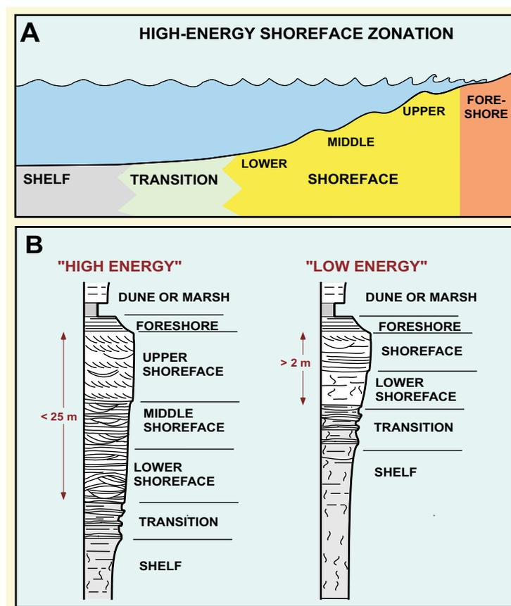
FIG. 3.—**A**) Beach-to-offshore profile (high-energy) in facies model of Galloway and Hobday (1996). Features a “transition zone” between shoreface and shelf. **B**) Shallowing-up facies succession in facies model of Galloway and Hobday (1996). Features a “transition zone” between shoreface and shelf in both high- and low-energy sequences.
