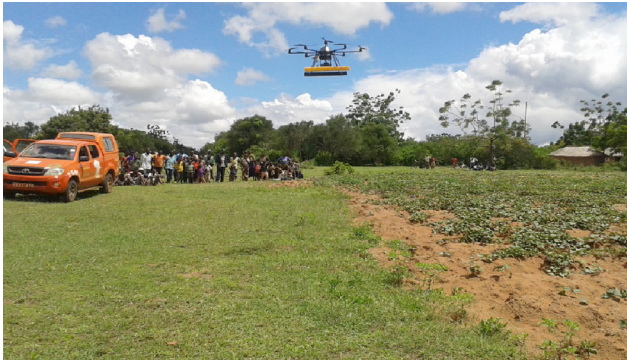
Fig. 3. Multirotor-based remote sensing system over farmers' fields in Tanzania. Photo courtesy of Roberto Quiroz, International Potato Centre.
