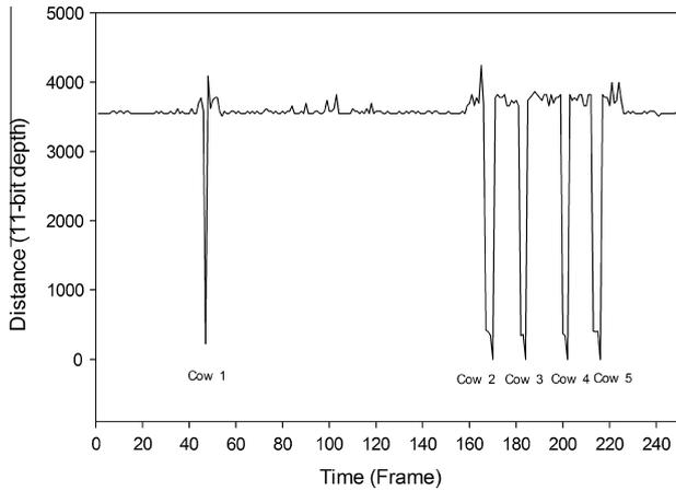
**Fig. 5.** Signal representing the distance from the object to the 3D camera sensor. Every minimum represents a cow passing through the sensor and it is used to automatically separate one cow from another.
