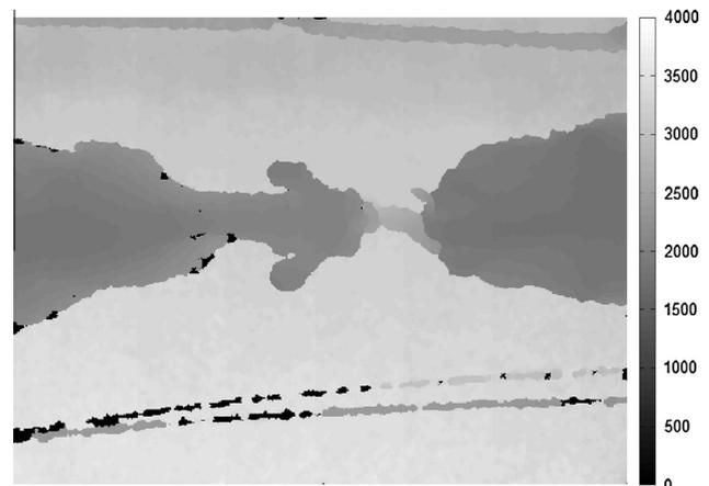
**Fig. 4.** Depth image extracted from the 3D camera, showing the cow traffic passing on the corridor. The pixel intensity represents the disparity matrix output of the 3D camera. The darker the pixels are the closer to the camera.
