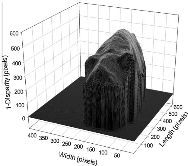
**Fig. 6.** Depth image after image segmentation reconstructed using mesh function in Matlab (2012b).
