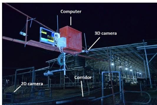
**Fig. 1.** Experimental setup. The corridor was built in order to force the cows to create a single file. The 3D camera was placed in top view of the corridor. The computer which the camera was connected to and where the videos were saved was placed in the box. The 2D camera was put on a tripod placed 6 m from the corridor perpendicular to the route of cow passage. Pictures were taken at night.
