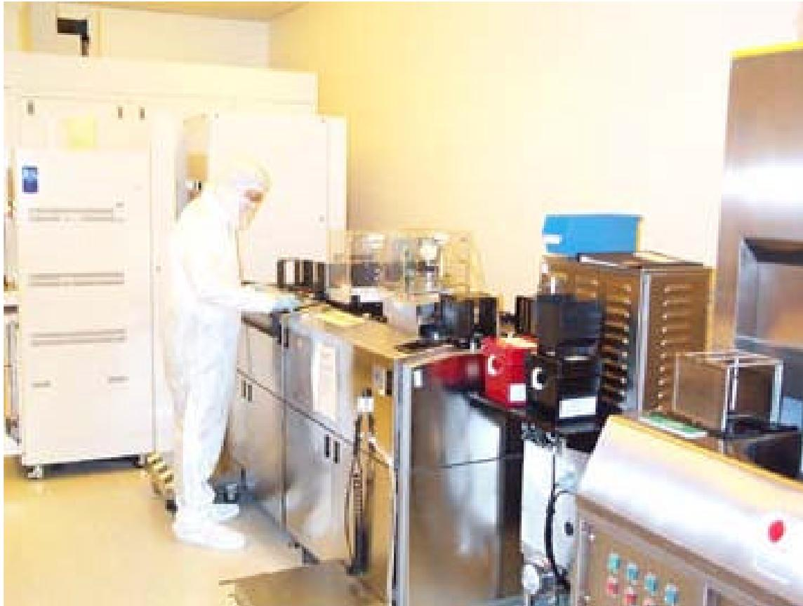
SSI coat and develop track
