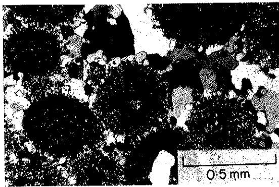
Fig. 9.11 Silicified oolite. Ooids have been replaced by microquartz and are enclosed in a megaquartz mosaic. Crossed polars. Cambrian. Pennsylvania, USA.
