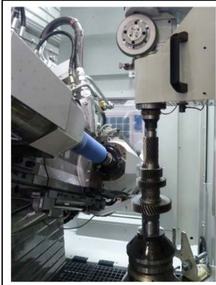
Figure 13 Drive shaft with asymmetric gear design.
