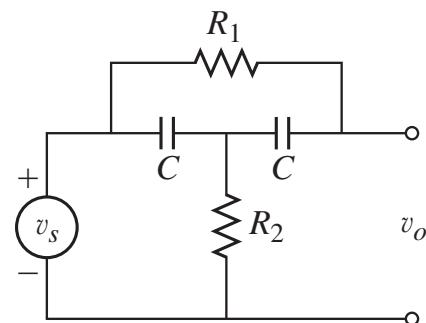
$$\frac{V_o(s)}{V_s(s)} = \frac{R_1R_2C^2s^2 + 2R_2Cs + 1}{R_1R_2C^2s^2 + (R_1 + 2R_2)Cs + 1}$$
