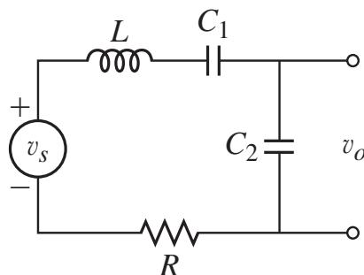
$$\frac{V_o(s)}{V_s(s)} = \frac{C_1s}{LC_1C_2s^3 + RC_1C_2s^2 + (C_1 + C_2)s}$$
