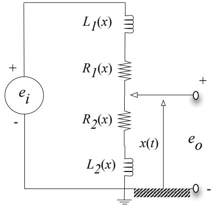
$$(L_1(x) + L_2(x)) \frac{di}{dt} + (R_1(x) + R_2(x)) i = e_i(t)$$
