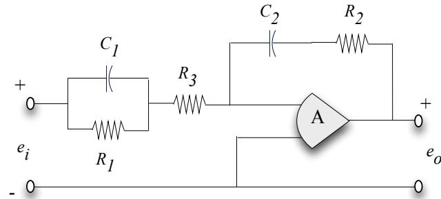
$$\frac{E_o(s)}{E_i(s)} = -\frac{(R_2 C_2 s + 1)(R_1 C_1 s + 1)}{C_2 s(R_3 R_1 C_1 s + R_3 + R_1)}$$
