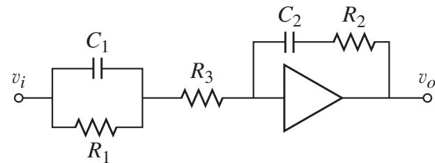
$$\frac{V_o(s)}{V_i(s)} = -\frac{R_3(R_1 C s + 1)}{R_1 R_2 C s + R_1 + R_2}$$
