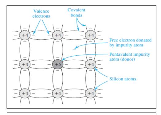
A silicon crystal doped by a pentavalent element. Each dopant atom donates a free electron and is thus called a donor. The doped semiconductor becomes *n* type.
