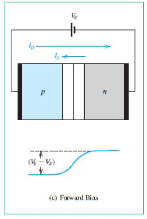
Here the applied voltage is in the direction that subtracts from the built-in voltage, resulting in a reduced barrier voltage across the depletion region.
