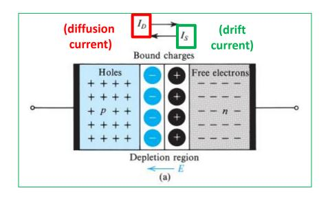
Under open-circuit conditions (Fig. 3.9) no external current exists; thus the two opposite currents across the junction must be equal in magnitude:
