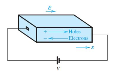
An electric field *E* established in a bar of silicon causes the holes to drift in the direction of *E* and the free electrons to drift in the opposite direction.
