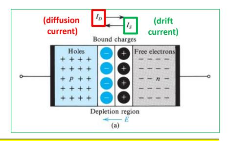
In addition to the current component  $I_D$  due to majority-carrier diffusion, a component due to minority carrier drift exists across the junction.
