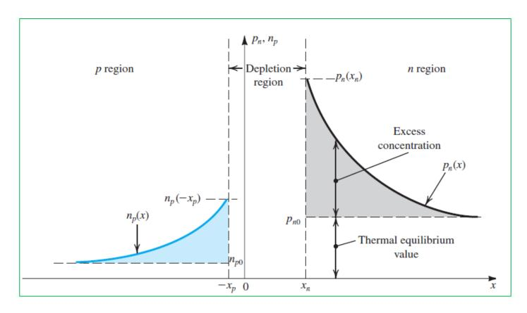
The excess hole charge stored in the *n* region can be found from the shaded area under the exponential as follows:
