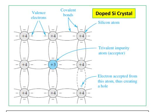
A silicon crystal doped with a trivalent impurity. **Each dopant atom gives rise to a hole**, and the semiconductor becomes **p** type.
