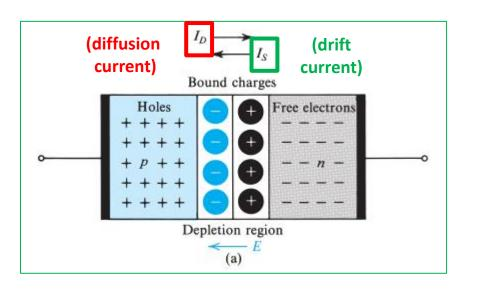
Because the concentration of holes is high in the p region and low in the n region, holes diffuse across the junction from the p side to the p side. Similarly, electrons diffuse across the junction from the p side to the p side. These two current components add together to form the diffusion current  $I_p$ , whose direction is from the p side to the p side.
