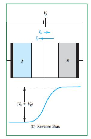
The externally applied reverse-bias voltage is in the direction to add to the barrier voltage, and it does, thus increasing the effective barrier voltage to  $(V_o + V_R)$  as shown in the equations below.
