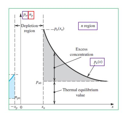
The exponential decay is characterized by the constant  $L_p$ , which is called the diffusion length of holes in the n material.
