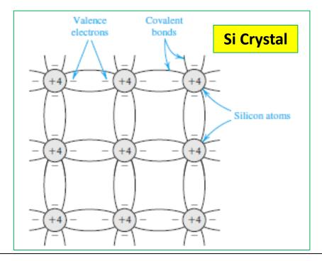
Two-dimensional representation of the silicon crystal. The circles represent the inner core of silicon atoms, with +4 indicating its positive charge of +4q, which is neutralized by the charge of the four valence electrons. Observe how the covalent bonds are formed by sharing of the valence electrons. At 0 K, all bonds are intact and no free electrons are available for current conduction.
