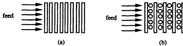
Fig. 2.25. Schematic drawing of a transversal flow module with fibers arranged parallel-in-line (a) and crossed-in-line (b).
