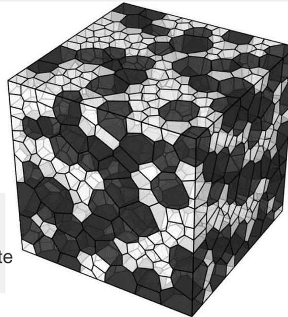
RVE with 6  $\mu\text{m}$  considering sphericity for ZTA 1, dark and white grains representing alumina and zirconia, respectively.
