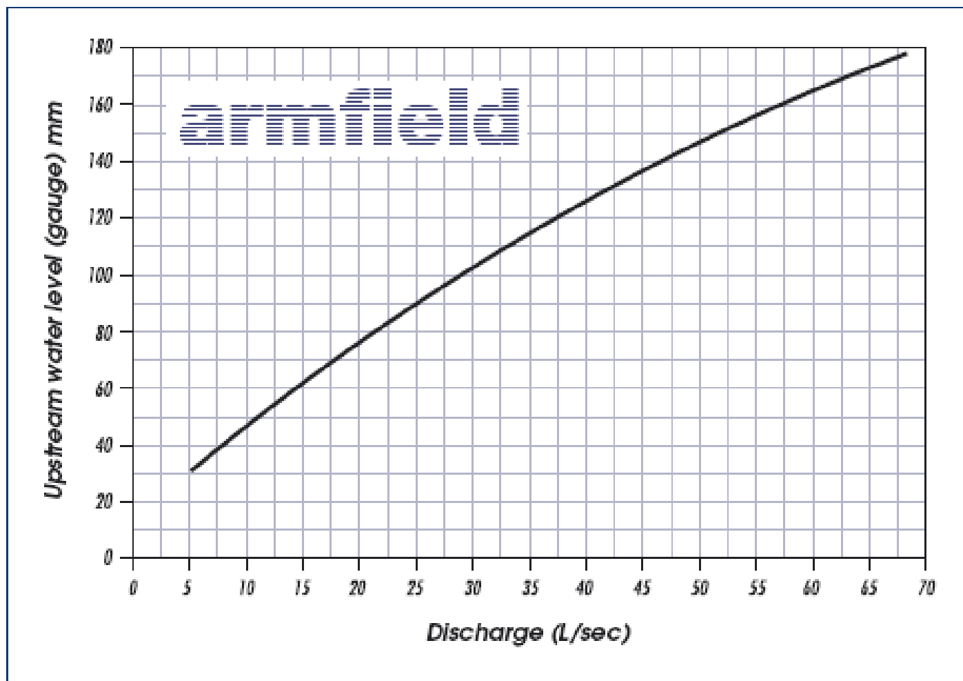
Calibration curve for a typical WSC flume
