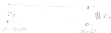
$$\frac{V}{I} = \frac{\frac{1}{2}(V_C + \sqrt{\frac{Z'}{Y'}} I_C) e^{\gamma x}}{\frac{1}{2} \left( \frac{V_C + \sqrt{\frac{Z'}{Y'}} I_C}{\sqrt{\frac{Z'}{Y'}}} \right) e^{\gamma x}} = \sqrt{\frac{Z'}{Y'}} \quad (1.27)$$
