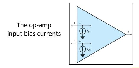
2 These two currents are represented by two current sources,  $I_{B1}$  and  $I_{B2}$ , connected to the two input terminals.
