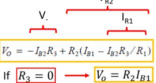
$$V_{O} = -I_{B2}R_{3} + R_{2}(I_{B1} - I_{B2}R_{3}/R_{1})$$
