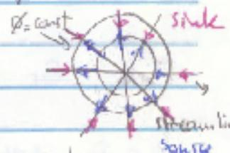
$\vec{r}$  refers to a point source at the origin. Whenever the source is placed anywhere else, we replace  $\vec{r}$  by the vector  $(\vec{r} - \vec{r}_0)$  where  $\vec{r}_0$  indicates the actual position of the source.
