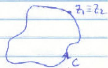
$$\Gamma + iQ = \oint_C W(z) dz = F(z_2) - F(z_1) \text{ where } z_1 \text{ and } z_2 \text{ are coincident points on } C$$
