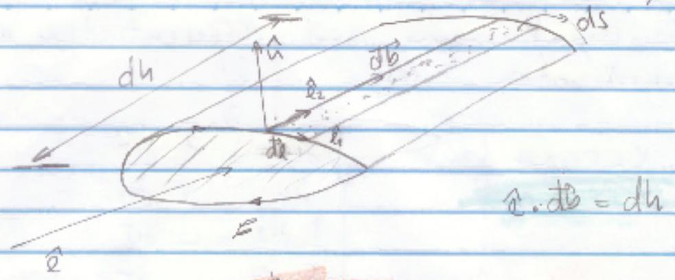
$$\rho \vec{U} \times \iint_S \hat{n} \times \vec{q} \, ds = \rho \vec{U} \times \int_{b_1}^{b_2} \Gamma(b) \hat{t} \, db \Rightarrow \text{Lift is related to circulation and vorticity!}$$
