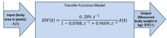
Fig. 5. The TF model adapted to estimate BW (in kg) using body area (in pixels) as input.
