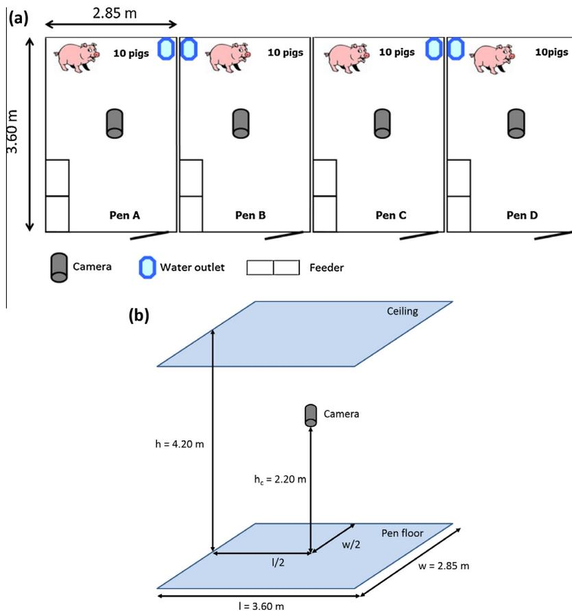
Fig. 1. (a) Ground plan of the 4 pens in the research barn; (b) position of the camera on top of a pen.
