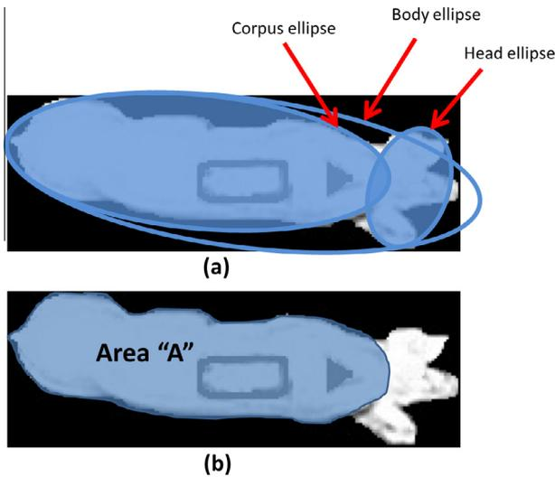
Fig. 3. (a) Extracted pig body using ellipse fitting; corpus and head separation by repeating ellipse fitting algorithm; (b) the resulting body area “A” used for BW estimation.
