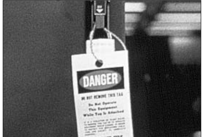
Turn off power, lock controls and tag
