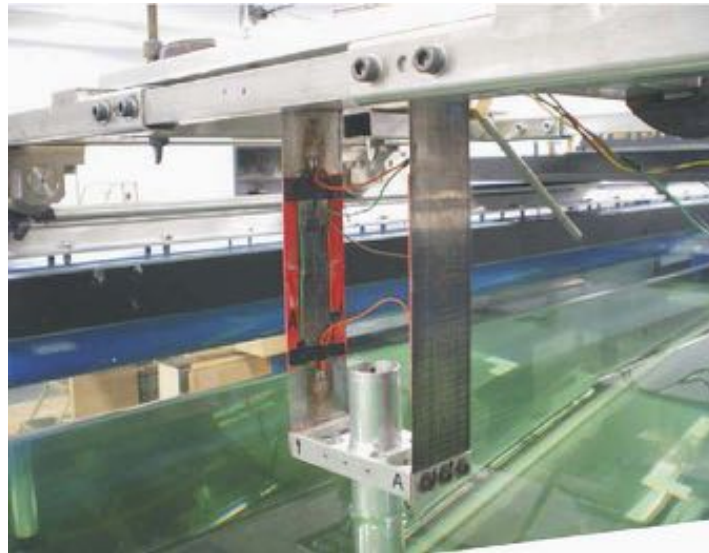
Fig. 4. Cylinder and elastic base mounted on the channel test-section structure.
