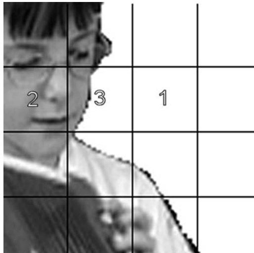
Figure 5.29 VO showing external (1), internal (2) and boundary (3) macroblocks
