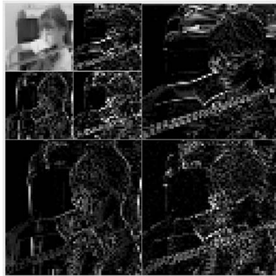
Figure 3.34 Two-stage wavelet decomposition of image
