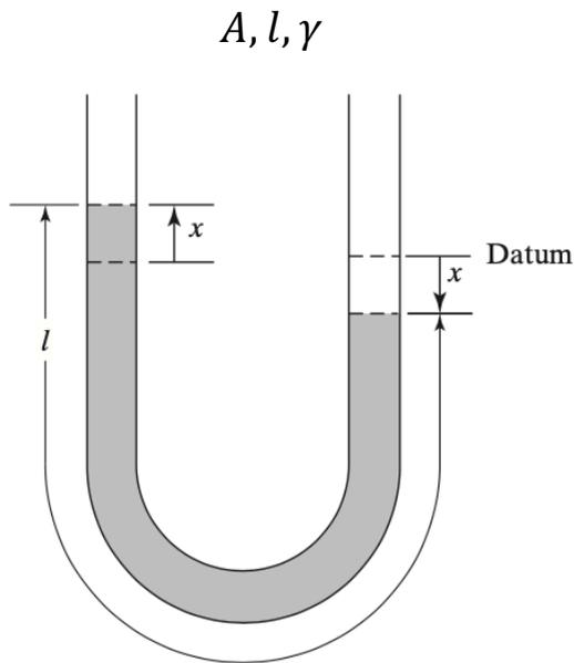
$$U = (Ax\gamma) \frac{x}{2} + (Ax\gamma) \frac{x}{2} = A\gamma x^2$$
