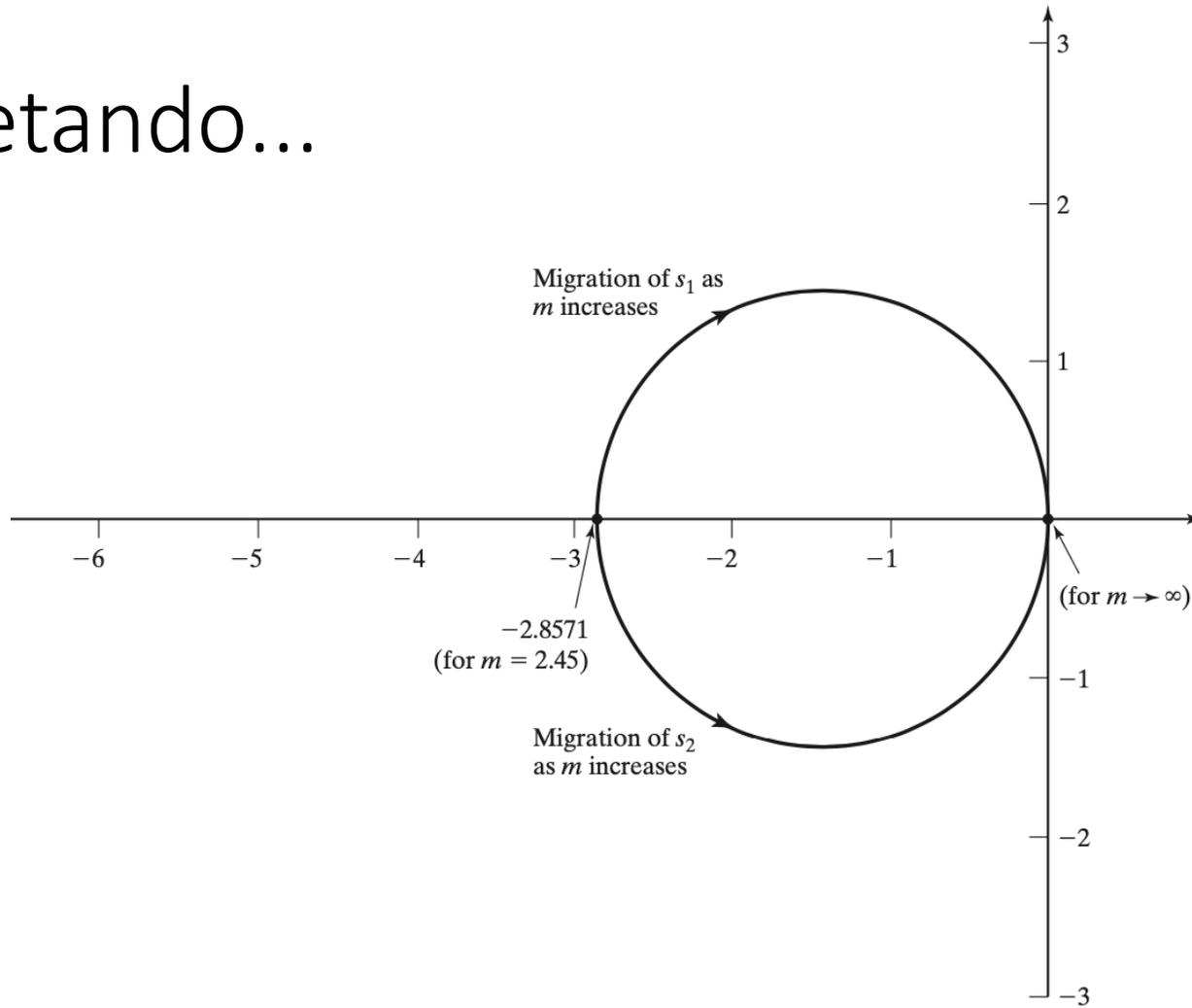
FIGURE 2.41 Root locus plot with variation of mass ( $m$ ).
