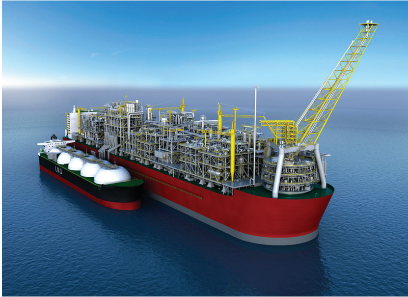
12.27 Model of floating liquefied natural gas factory (Shell Prelude)
