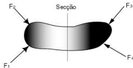
$$\Sigma F=0 \rightarrow \Sigma F_x=0; \Sigma F_y=0; \Sigma F_z=0$$
