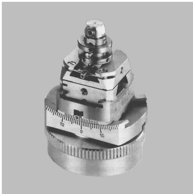
Figure 1.11. A goniometer head.
