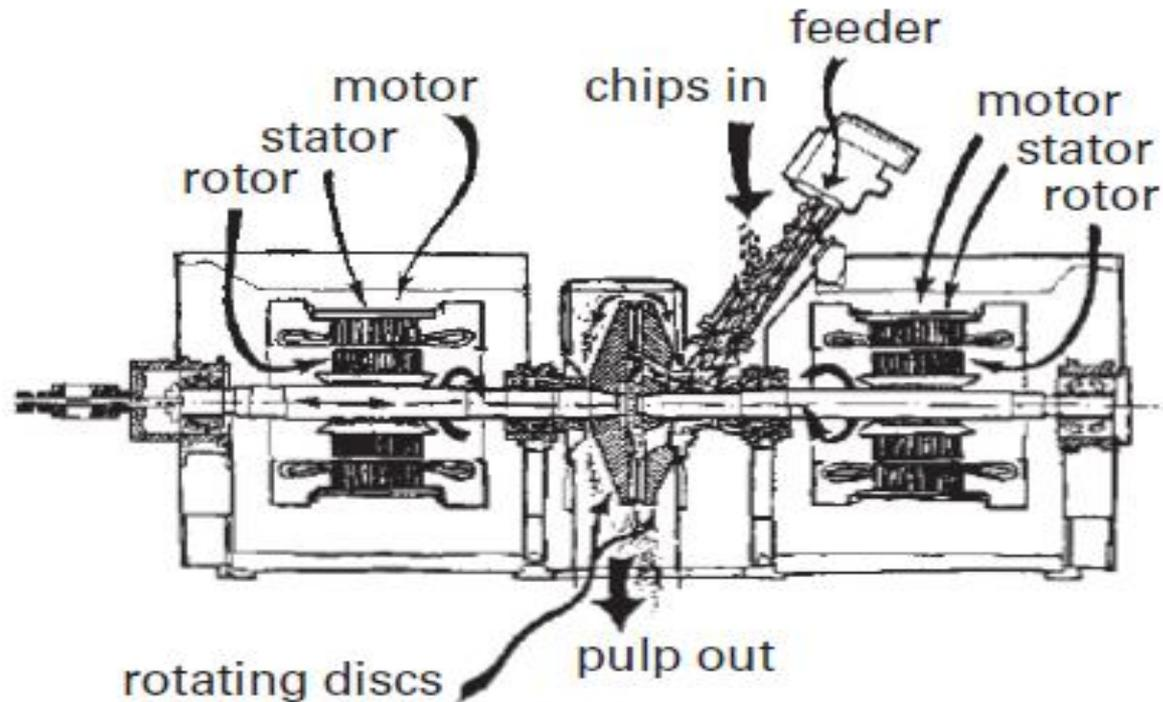
**Figure 4.2.** Double disc refiner.
