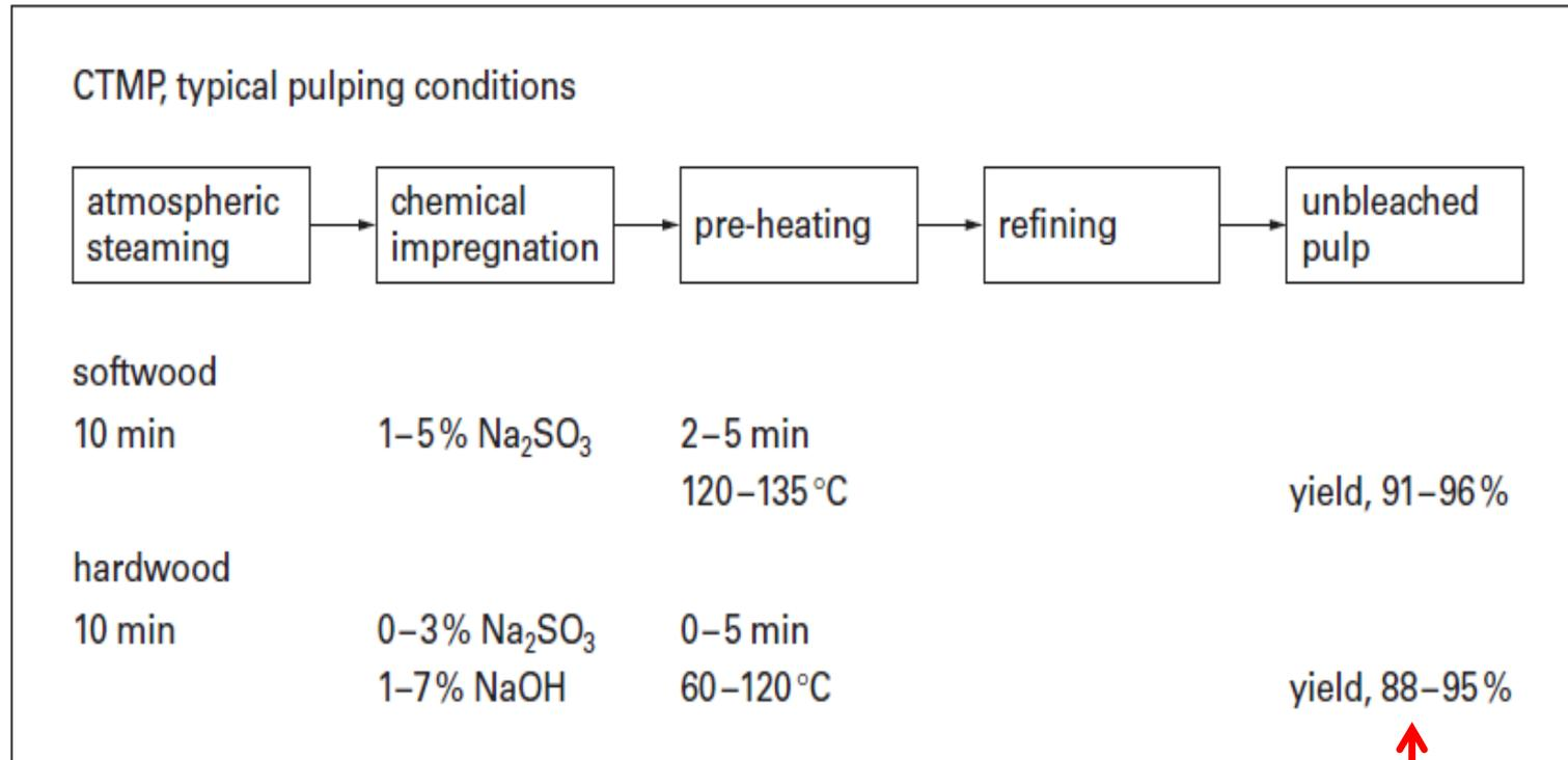
Figure 4.29. Unit operations in typical CTMP processes.
