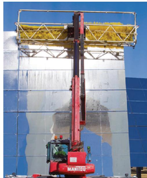
Figure 41: Abengoa truck with mirror cleaning equipment [38]
