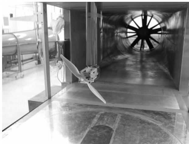
Figure 2.2: Photograph of test section with experimental rig installed.
