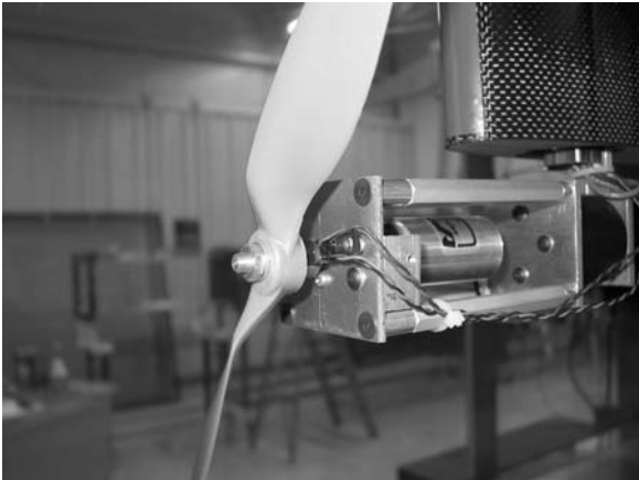
Figure 2.7: Photoreflector aimed at the output shaft.
