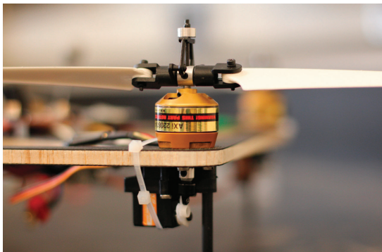
(a) Variable-pitch actuator
