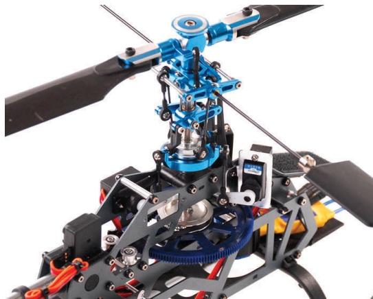
(b) RC helicopter swashplate
