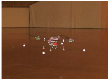
Figure 4.19: OS4 in hover. A training frame was added for safety.
