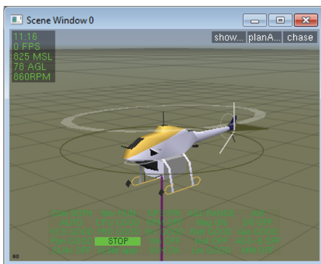
Figure 9.5-5 Visualization of Yamaha RMAX in simulation environment.
