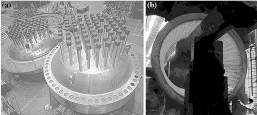
**Fig. 3.2** Reactor pressure vessel head and ring forging procedure. **a** Reactor Pressure vessel head (Source [1], US-NRC) **b** Ring forging process (Source [2], Doosan Heavy)
