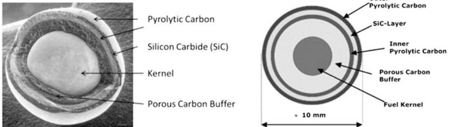
**Fig. 3.11** TRISO coated fuel particle. **a** (V)HTR fuel [71]. **b** Schematic drawing of a TRISO coated particle
