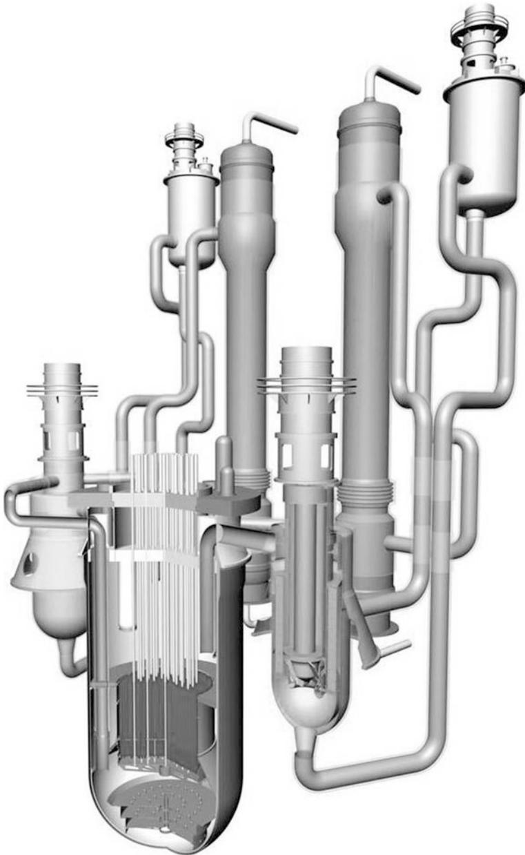
**Fig. 3.5** Japanese sodium fast reactor (JSFR) reactor vessel and internal structures (*Source* [49], copyright: JAEA-Research 2006-042)
