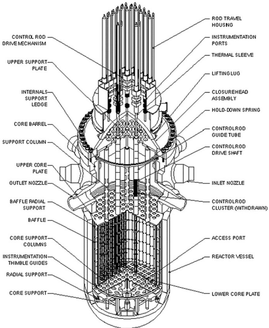
**Fig. 3.1** Cut through a pressure vessel of a pressurized light water reactor (Source [47])
