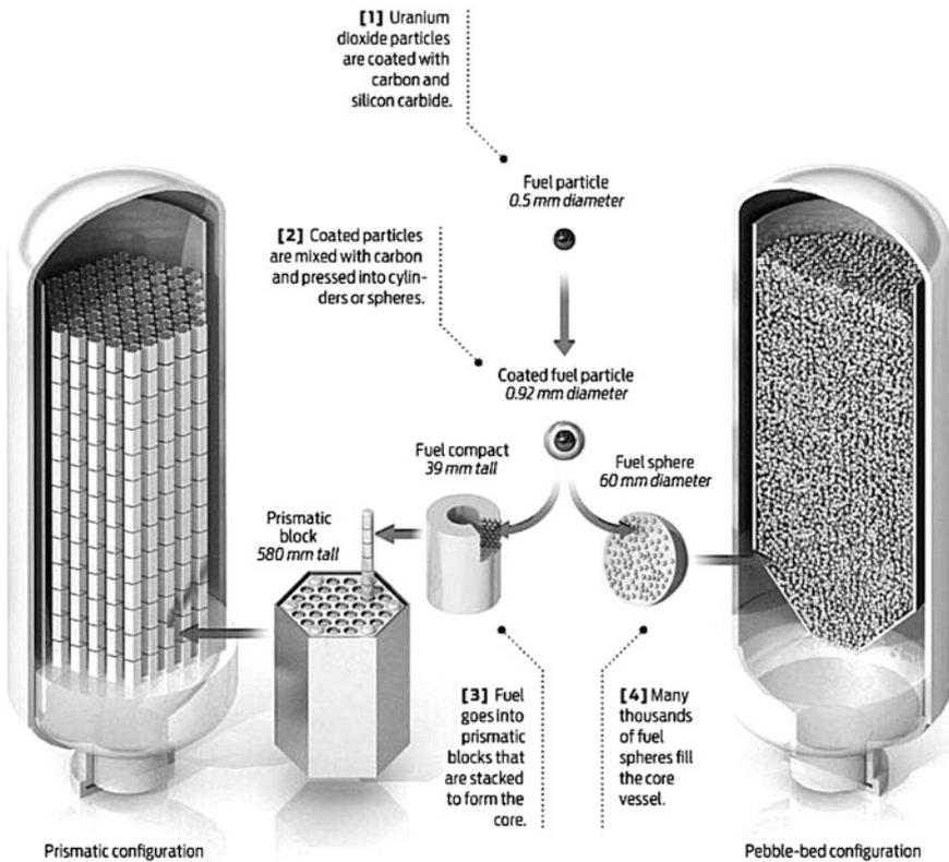
**Fig. 3.12** The two options for a high temperature gas reactor (HTR). (Copyright: Artwork by Bryan Christie)
