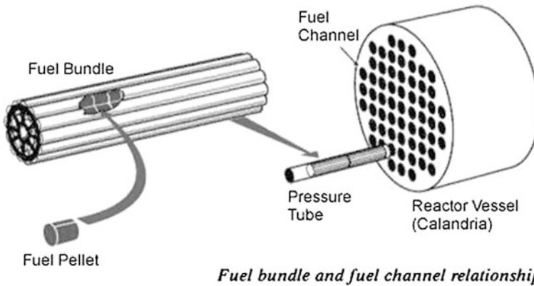
**Fig. 3.7** Sketch of the fuel arrangement in a CANDU-reactor. The pressure tubes fit into the channels of the Calandria which acts as pressure vessel [5]
