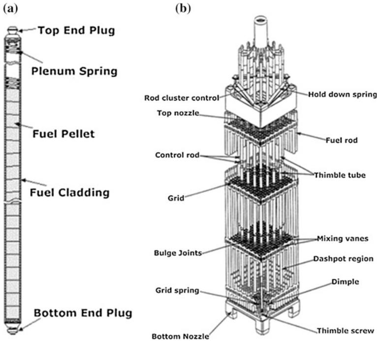
**Fig. 3.6** Fuel pin and fuel assembly of a light water reactor. **a** Fuel pin of a light water reactor. **b** Fuel assembly of a light water reactor (Source [70])
