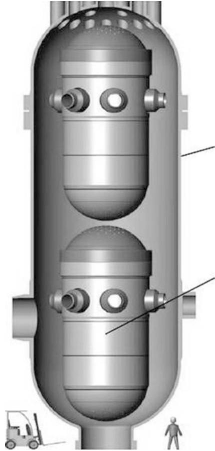
steel) type material can be used as a cold vessel option. However, more advanced, future concepts will operate at higher metal temperatures in the creep regime and consequently a reconsideration of 9Cr-1Mo needs to be done. One of the major problems of the HTR vessel is its huge dimension which is shown in Fig. 3.3.
