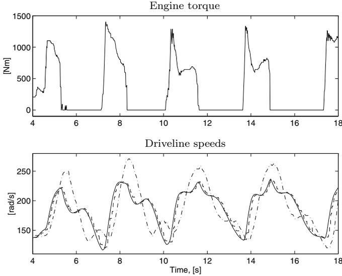
**Figure 7.7** Logged data on the CAN-bus during step inputs in accelerator position with the 144L truck. The transmission speed (dashed) and the wheel speed (dash-dotted) are scaled to engine speed in solid. The main flexibility of the driveline is located between the output shaft of the transmission and the wheel, since the largest difference in speed is between the measured transmission speed and wheel speed.
