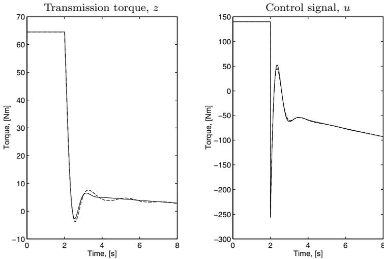
**Figure 7.61** Simulation of the Nonlinear clutch and drive-shaft model with observer and control law based on the Drive-shaft model. A gear shift is commanded at  $t=2$  s. Feedback from the wheel-speed sensor is shown in solid lines, and feedback from the engine-speed sensor is shown in dashed lines. The design still works when simulated with extra clutch dynamics.
