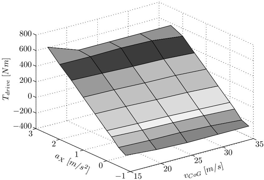
**Figure 11.26** Drive torque of the engine as a function of acceleration and velocity
