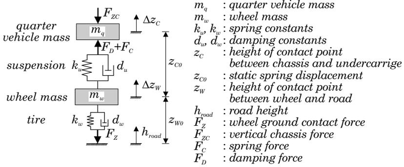
Figure 8.26 Forces and displacements in the quarter vehicle model
