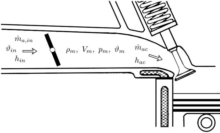
**Figure 3.17** Cross-section of intake manifold
