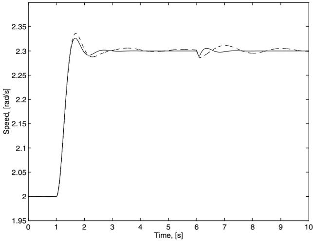
**Figure 7.47** Wheel-speed response of step in accelerator position at  $t=1$  s with the speed controller (7.141) derived from the Drive-shaft model, controlling the Nonlinear clutch and drive-shaft model. The solid line corresponds to  $\dot{\alpha}_w$ -feedback and feedback from  $\dot{\alpha}_{CS}$  is seen in dashed line. At  $t=6$  s, an impulse disturbance  $v$  acts on the load. The design still works when simulated with extra clutch dynamics.
