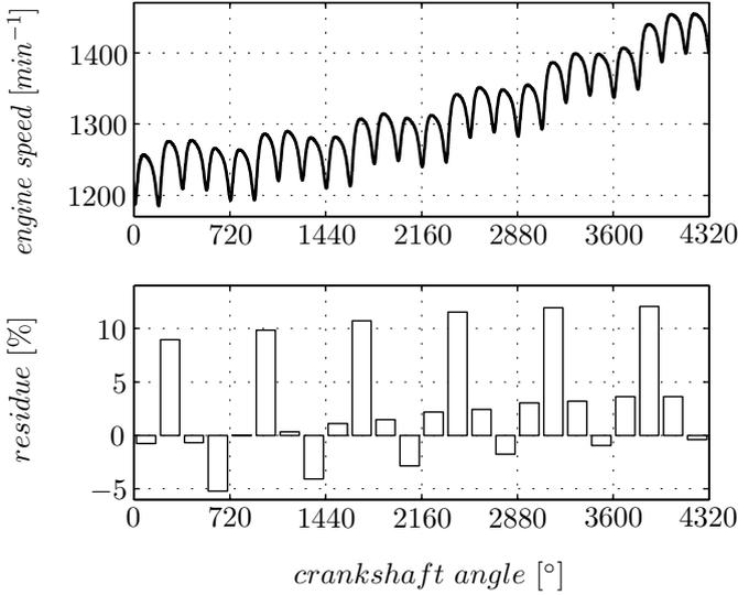
**Figure 5.47** Uncompensated residues at 4-cylinder engine during transient
