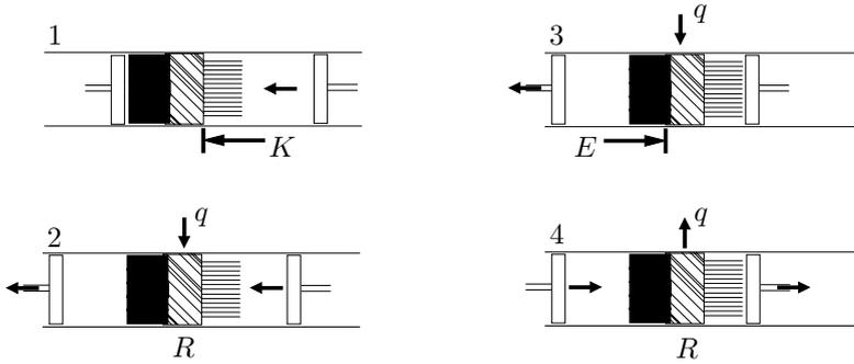
**Figure 2.21** The four steps of the Stirling cycle
