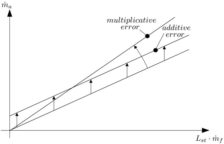
**Figure 5.21** Simplified error model for the lambda characteristic
