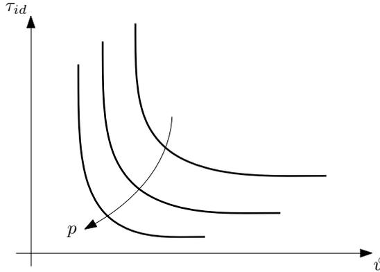
**Figure 3.7** Delay of self-ignition  $\tau_{id}$  over temperature  $\vartheta$  for different pressure values  $p$ .
