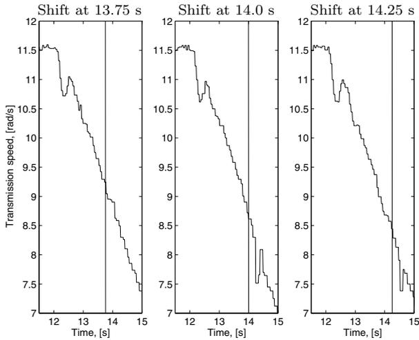
**Figure 7.67** Same type of field experiment as in Figure 7.65, but with commanded engagement of neutral gear at 13.75, 14.0, and 14.25 s. The amplitudes of the transmission speed oscillations after the gear shift are less than 1 rad/s with different signs, which is an acceptable level.
