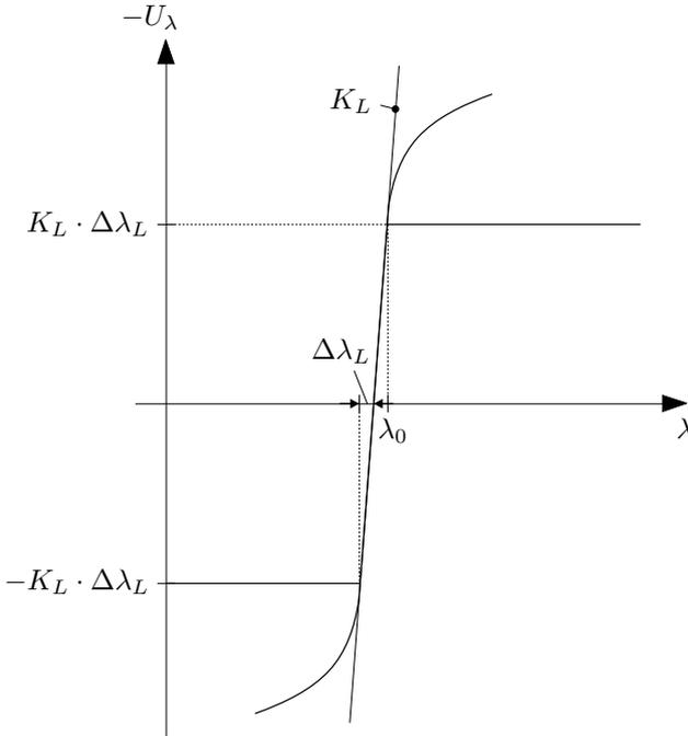
**Figure 5.12** Inverted  $\lambda$ -characteristic with limiting range  $\pm\Delta\lambda_L$
