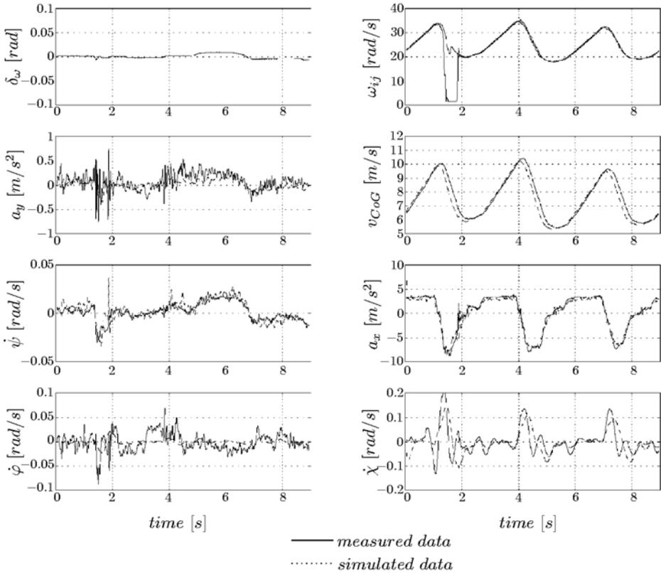
**Figure 8.32** Model validation: straight ahead braking and acceleration
