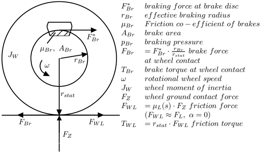
Figure 10.1 Torque balance at the wheel-road surface contact
