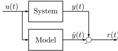
**Figure 6.6** Simple fault detection system
