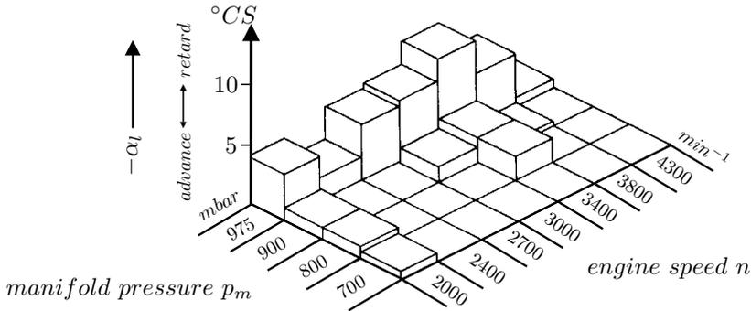
**Figure 5.44** Adaptation of ignition angle map  $\alpha_i$  after 50 km ride, 50 : 50 mixture of 91 and 98 octane fuel.
