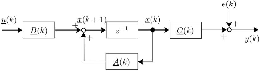
**Figure 9.3** Velocity estimation using a Kalman Filter
