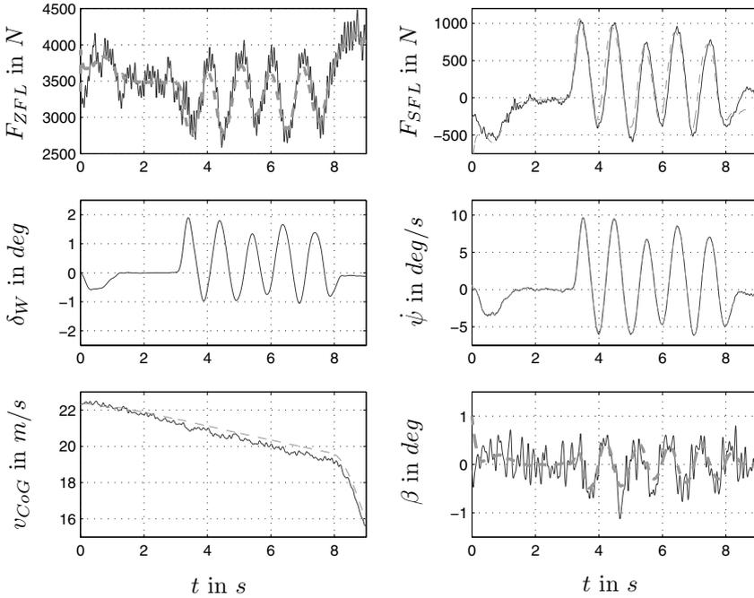
**Figure 9.44** Validation of vehicle body side slip angle observer with a sinusoidal test drive
