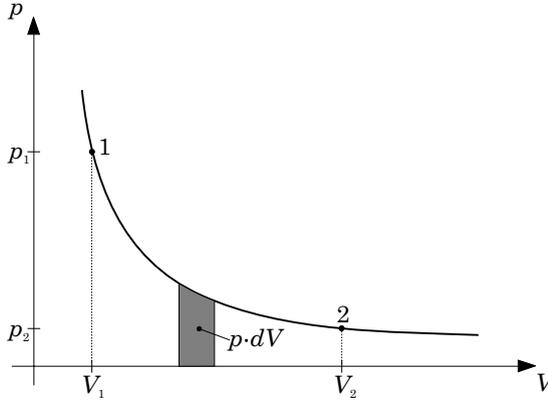
**Figure 2.1** Mechanical work due to volume change.
