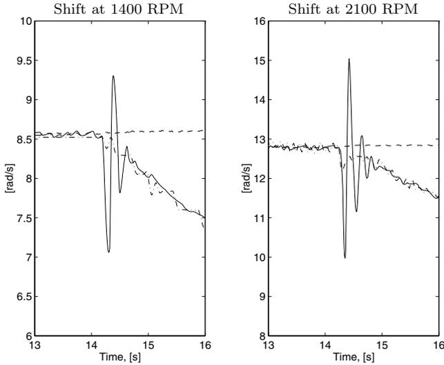
**Figure 7.21** Engagement of neutral gear commanded at 14 s, with stationary driveline at 1400 RPM and 2100 RPM on a flat road with gear 1. Engine speed (dashed) and wheel speed (dash-dotted) are scaled to transmission speed which is seen in solid lines. After a delay time, neutral gear is engaged, causing the driveline speeds to oscillate. The amplitude of the oscillating transmission speed is higher the higher the speed is.
