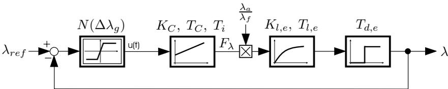
**Figure 5.13** Closed loop-control circuit of the lambda-control
