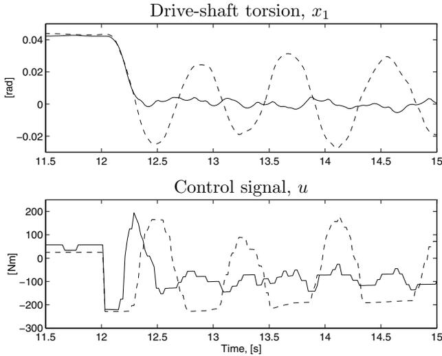
**Figure 7.64** Control signal and drive-shaft torsion when using the gear-shift controller that controls the drive-shaft torsion to zero, started at 12.0 s. Prior to that, the engine has the stationary speed 1900 RPM with gear 1 engaged. In dashed lines, a PI controller is used that gives  $x_1 = 0$ , but with undamped driveline resonances. The solid lines are extension with the active damping controller.
