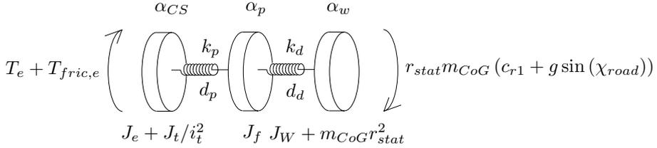
**Figure 7.11** Model with flexible propeller shaft and drive shaft.
