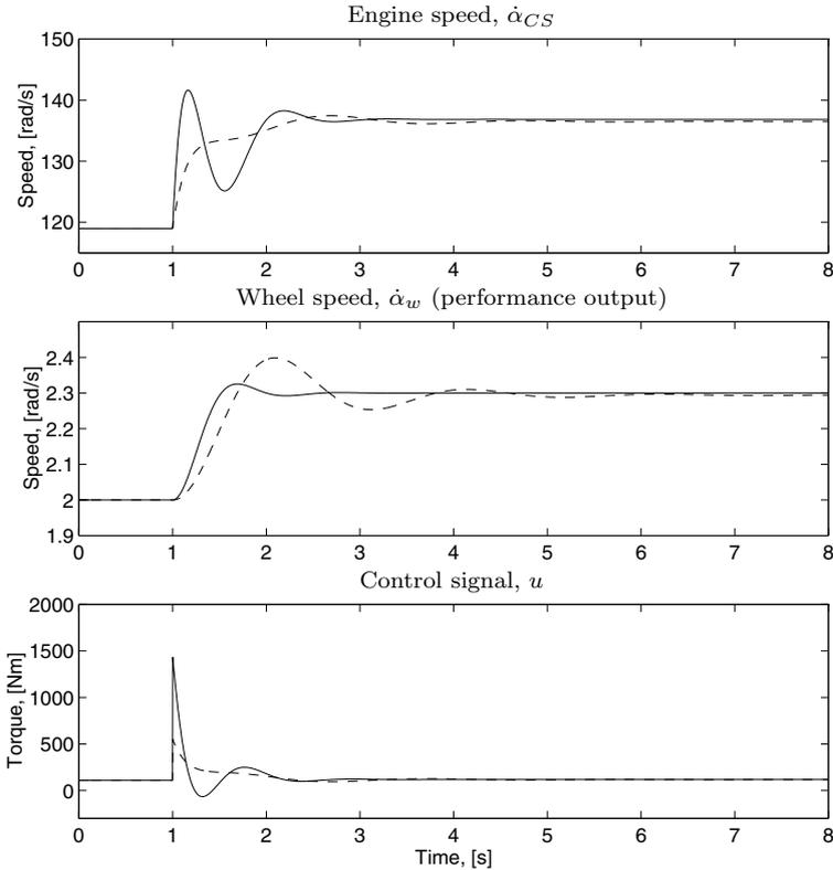
**Figure 7.40** Response of step in accelerator position at  $t=1$  s. The Drive-shaft model is controlled with the speed control law (7.139) in solid lines. RQV control (7.115) with  $K_p=25$  is seen in dashed lines. With active damping, the engine speed oscillates, resulting in a well damped wheel speed.
