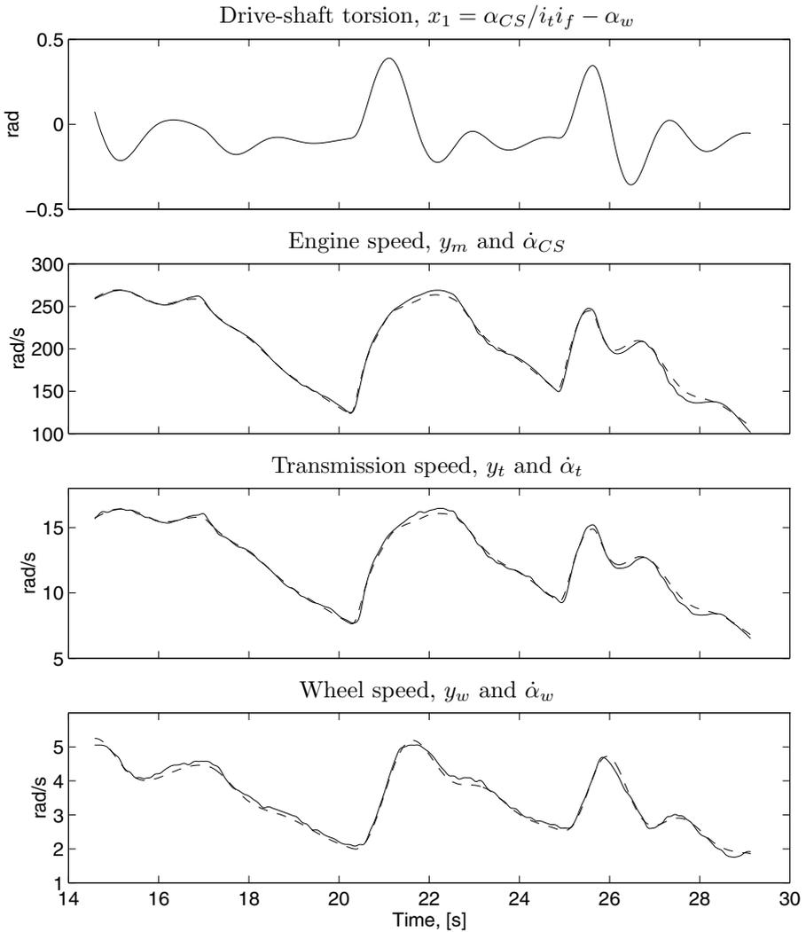
**Figure 7.14** Parameter estimation of the Drive-shaft model as in Figure 7.10, but with sensor dynamics included. The top figure shows the estimated drive-shaft torsion, and the bottom figures show the model outputs ( $y_m, y_t, y_w$ ) in dashed, together with the measured data in solid. The main part of the deviation between engine speed and transmission speed is due to sensor dynamics. See also Figure 7.15.
