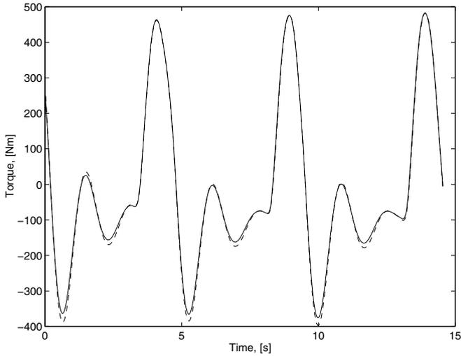
**Figure 7.52** Estimated transmission torque,  $z$ , in (7.175) and (7.192) for a test with step inputs in accelerator position with the 144L truck. The solid line corresponds to the Drive-shaft model and the dashed line corresponds to the Clutch and drive-shaft model.
