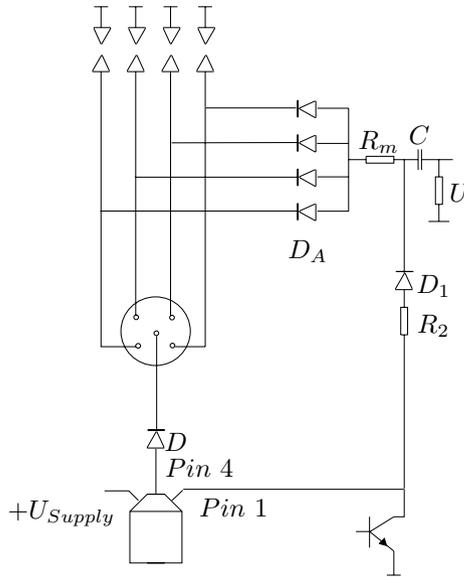
**Figure 5.36** Ion current measurement via high voltage diodes
