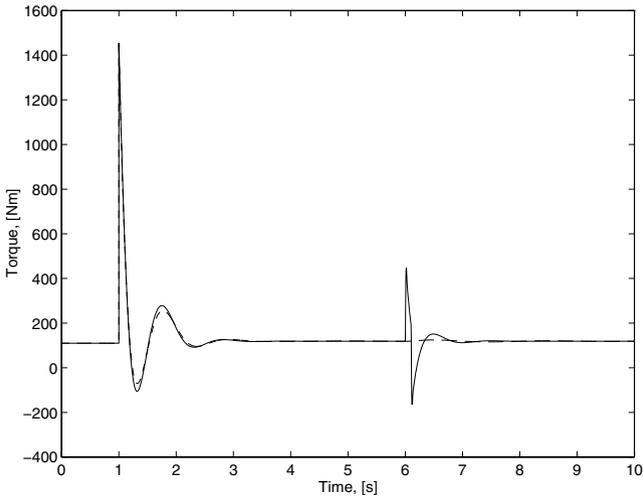
**Figure 7.48** Control signal corresponding to Figure 7.47. There is only little difference between the two sensor alternatives in the step response at  $t=1$  s. However, the load impulse (at  $t=6$  s) generates a control signal that damps the impulse disturbance when feedback from the wheel-speed sensor is used, but not with engine-speed feedback.
