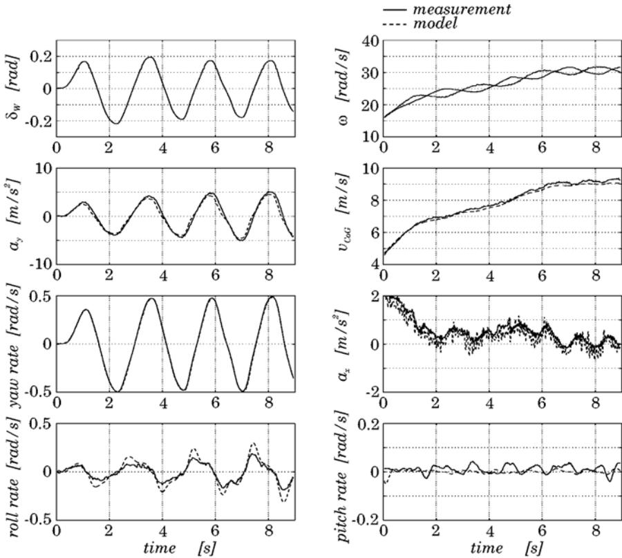
Figure 8.34 Model validation: sine wave form steering
