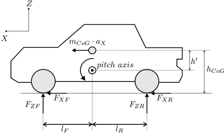
**Figure 9.28** Torque balance at the pitch axis
