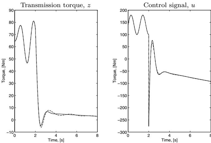
**Figure 7.62** Same simulation case as in Figure 7.61, but with driveline oscillations at the start of the transmission-torque controller. Feedback from the wheel-speed sensor is shown in solid lines, and feedback from the engine-speed sensor is shown in dashed lines. The conclusion is that the control law works well despite initial driveline oscillations.
