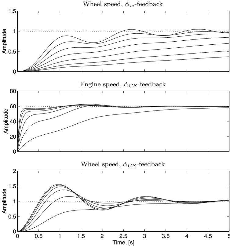
**Figure 7.32** Step responses when using a P-controller with different gains on the Drive-shaft model with gear 1. With  $\dot{\alpha}_w$ -feedback (top figure), increased gain results in instability. With  $\dot{\alpha}_{CS}$ -feedback (bottom figures), increased gain results in a well damped engine speed, but an oscillating wheel speed.
