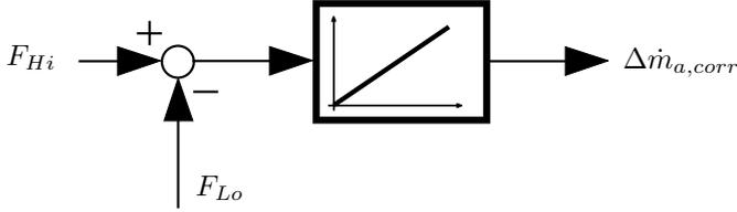
**Figure 5.22** Additional integral controller for offset correction
