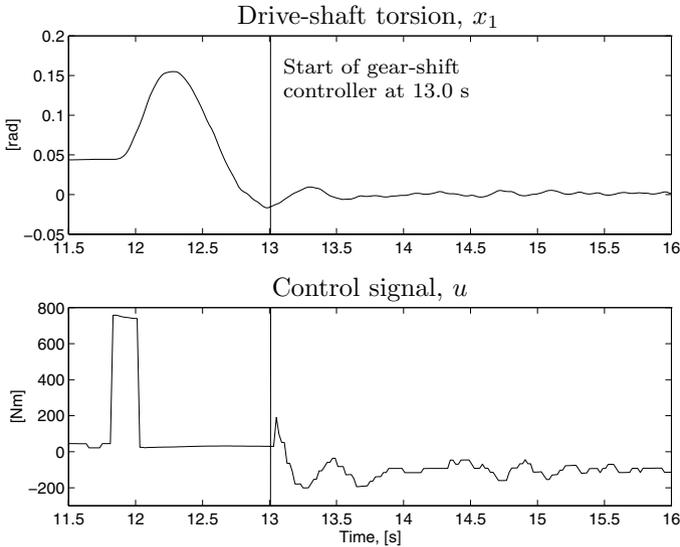
**Figure 7.68** Control signal and drive-shaft torsion during field trials with start of the gear-shift controller at 13.0 s. The driveline is oscillating prior to the gear shift due to an engine torque pulse at 11.7 s. The controller controls the drive-shaft torsion to zero with damped resonances despite initial driveline oscillations.
