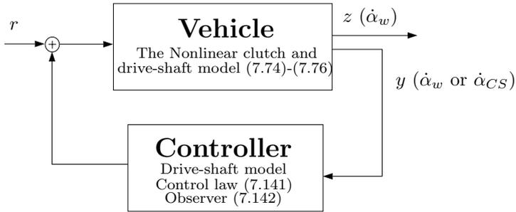
**Figure 7.46** Simulation configuration. As a step for demonstrating feasibility for real implementation, the Nonlinear clutch and drive-shaft model is simulated with the controller based on the Drive-shaft model.
