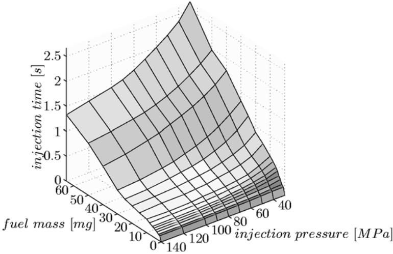
**Figure 3.15** Piezoelectric injector map ( $1\text{MPa} = 10\text{bar}$ )
