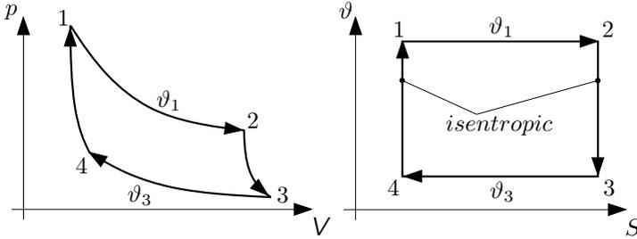
**Figure 2.9**  $pV$ -diagram and  $\vartheta S$ -diagram of Carnot Cycle.
