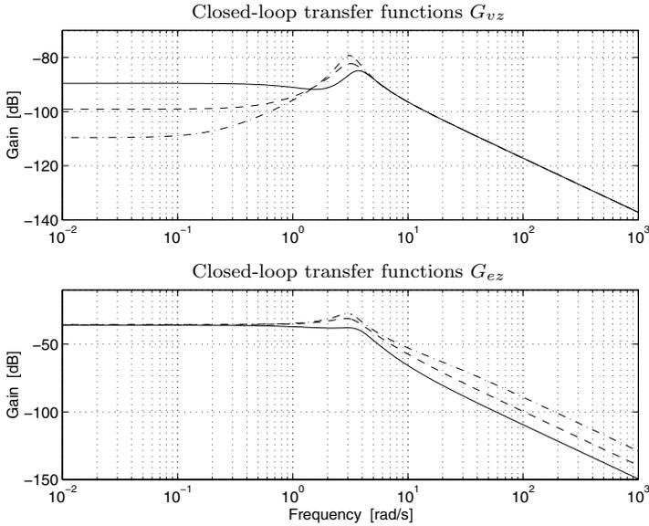
**Figure 7.38** Closed-loop transfer functions  $G_{vz}$  and  $G_{ez}$  when using the RQV control law (7.115) for the controller gains  $K_p=8$  (solid),  $K_p=25$  (dashed), and  $K_p=85$  (dash-dotted). The resonance peaks increase with increasing gain.
