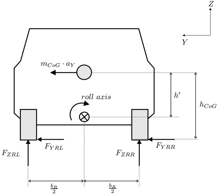
Figure 9.27 Torque balance at the roll axis
