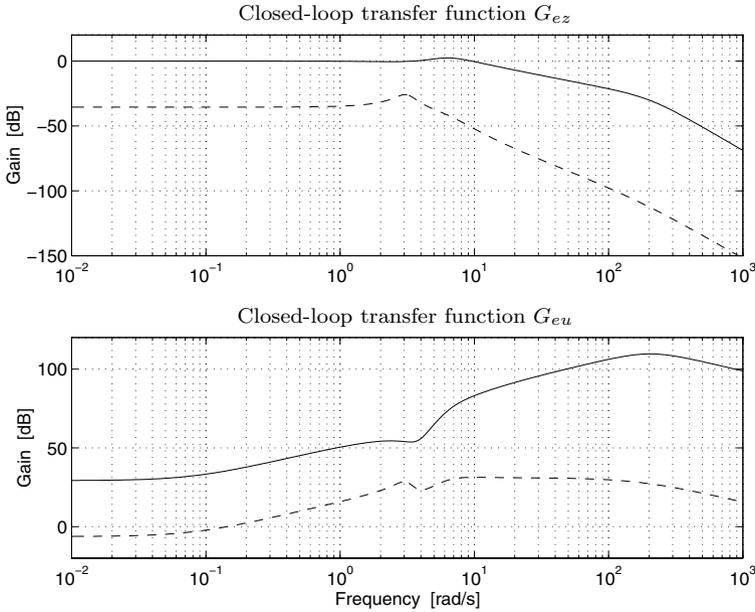
**Figure 7.43** Closed-loop transfer functions from measurement noise,  $e$ , to performance output,  $z$ , and to control signal,  $u$ . Feedback from  $\dot{\alpha}_w$  is shown in solid and feedback from  $\dot{\alpha}_{CS}$  is shown in dashed lines. The difference between the two feedback principles is described by the dynamic output ratio. The effect increases with lower gears.
