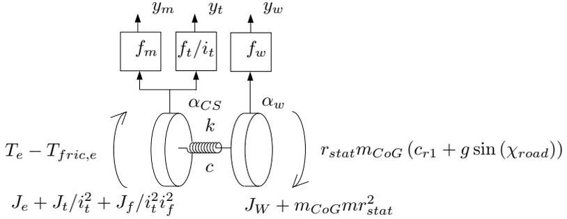
**Figure 7.13** The Drive-shaft model with sensor dynamics.
