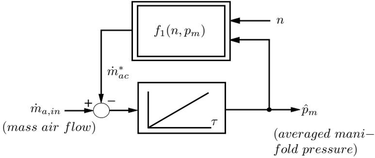
**Figure 3.18** Dynamic model of intake manifold
