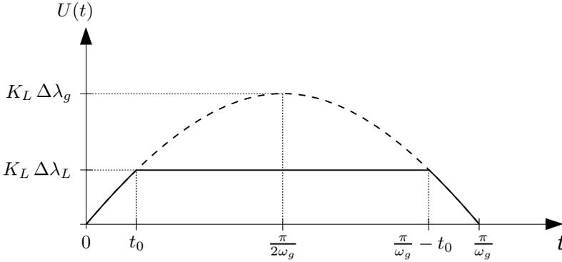
**Figure 5.14** Limiting of the output sine function  $U(t)$
