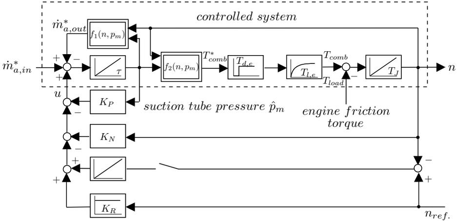
**Figure 5.27** Block diagram of idle speed control
