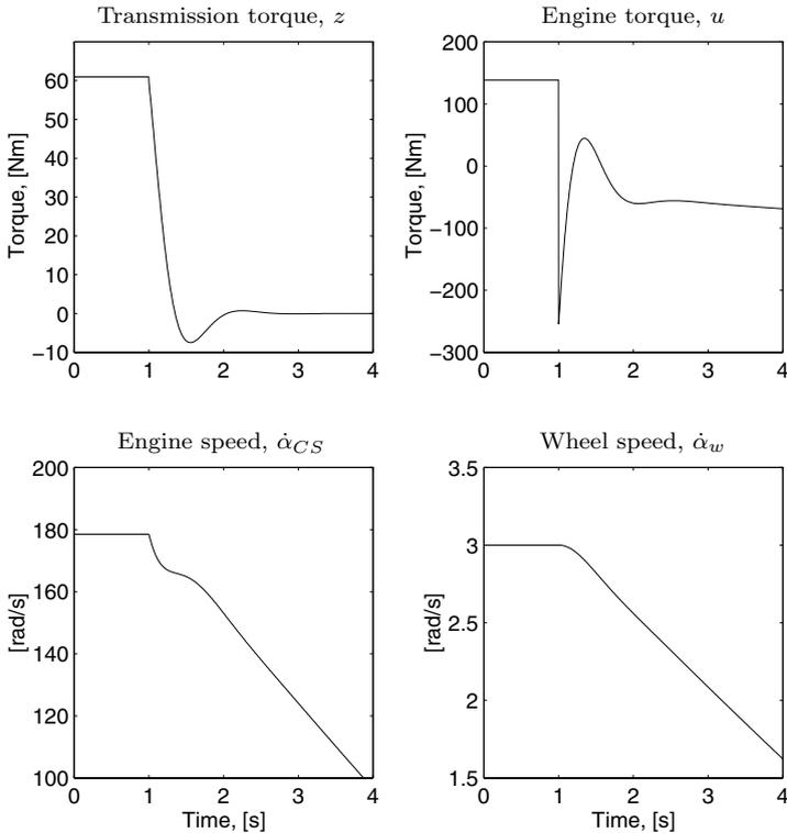
**Figure 7.56** The Drive-shaft model controlled with the transmission-torque controller (7.219), solving the gear-shift criterion (7.209). At  $t=1$  s, a gear shift is commanded. A realizable control signal is used such that the transmission torque is driven to zero, while oscillations are actively damped.
