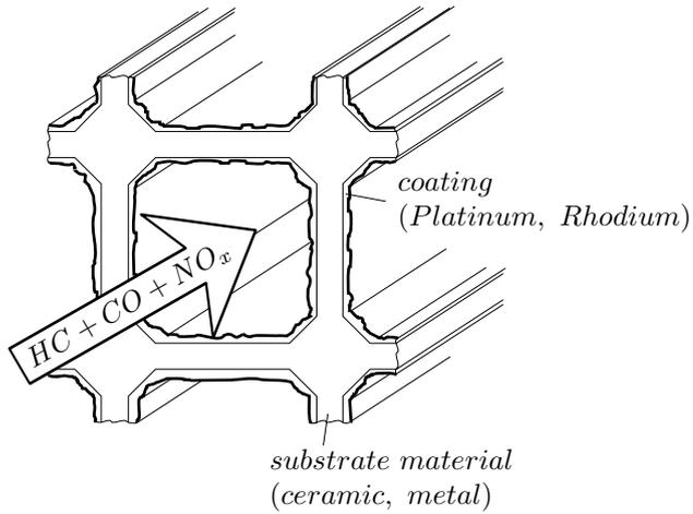
**Figure 5.4** Exploded view of a catalytic converter.
