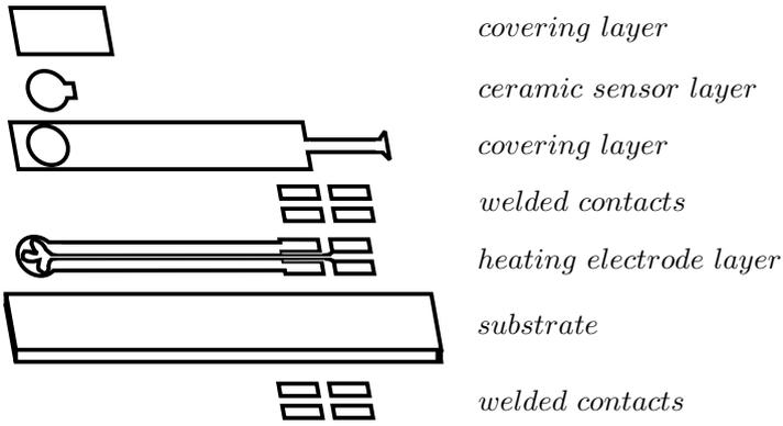
**Figure 5.7** Planar structure of the strontium titanate sensor
