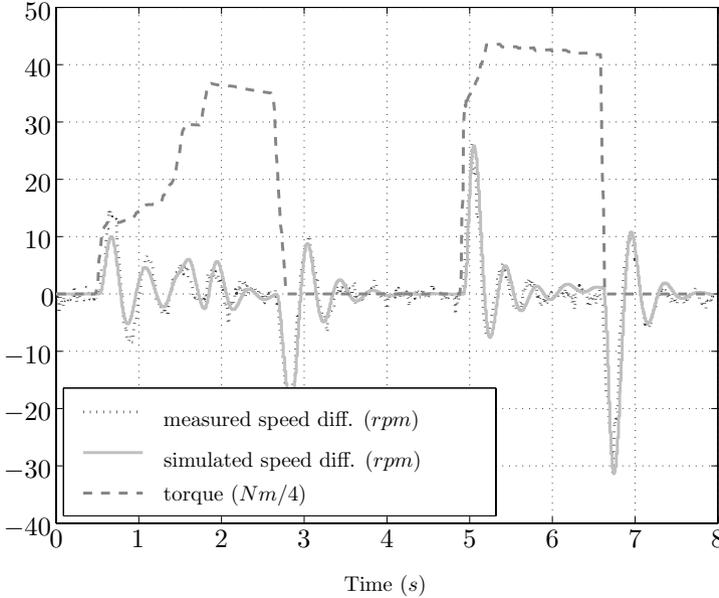
**Figure 7.73** Measured and Simulated Speed Difference
