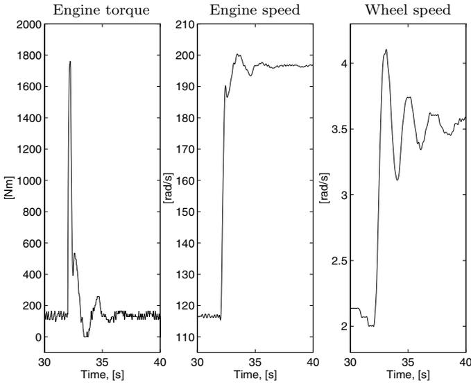
**Figure 7.27** Measured speed response of a step in accelerator position at  $t=32$  s. An RQV speed controller controls the engine speed to 2000 RPM. The engine speed is well damped, but the resonances in the driveline is seen to give oscillating wheel speed, resulting in vehicle shuffle.
