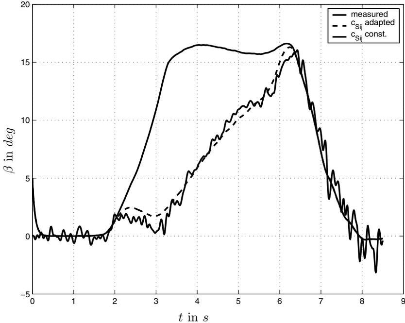
**Figure 9.43** Observed vehicle body side slip angle with and without adaptation of the tire side slip constants
