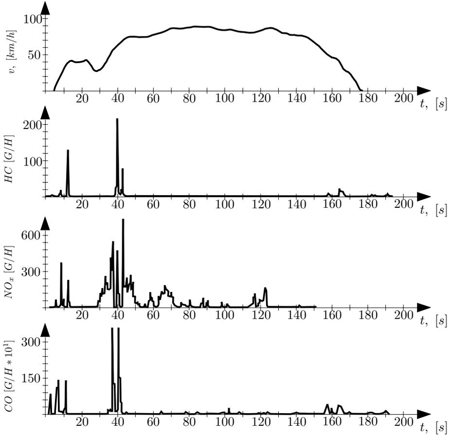
**Figure 5.19** Emissions of lambda-controlled engine after catalytic conversion, FTP-HT2 driving-cycle
