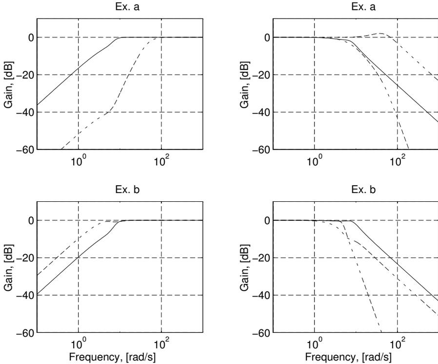
**Figure 7.34** Closed-loop transfer functions  $S$  (left figures), and  $T$  (right figures). Feedback from  $\dot{\alpha}_w$  is seen in solid lines, and feedback from  $\dot{\alpha}_{CS}$  in dashed lines.  $\overline{T}_m$  is seen in the right figures in dash-dotted lines. For the  $\dot{\alpha}_{CS}$ -design,  $W = 5 \cdot 10^4$  (Ex. 7.1a) and  $W = 50$  (Ex. 7.1b) are used, and for the  $\dot{\alpha}_w$ -design,  $W = 15$  (Ex. 7.1a) and  $W = 5 \cdot 10^2$  (Ex. 7.1b) are used.
