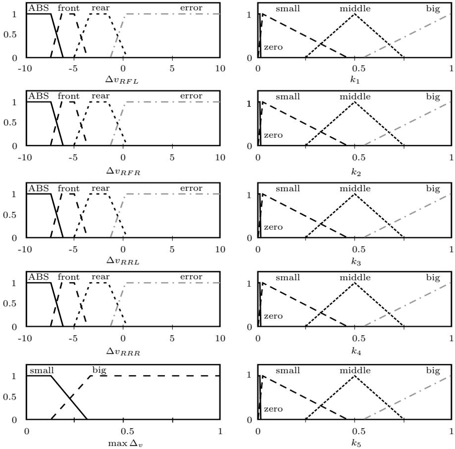
**Figure 9.8** Membership functions of sub-system "strong Braking"
