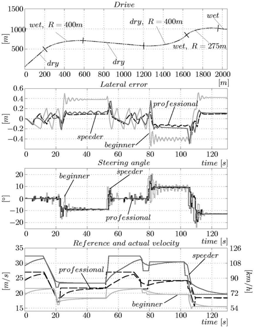
Figure 11.34 Lateral controller with different drivers
