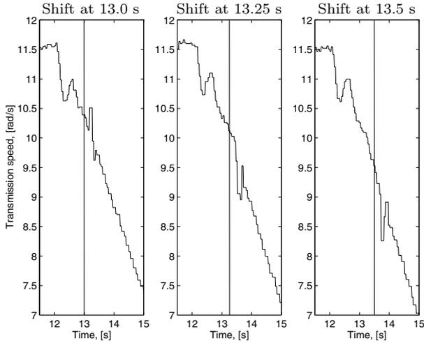
**Figure 7.66** Same type of field experiment as in Figure 7.65, but with commanded engagement of neutral gear at 13.0, 13.25, and 13.5 s. The amplitudes of the transmission speed oscillations after the gear shift are less than 1 rad/s with different signs, which is an acceptable level.
