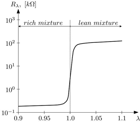
**Figure 5.8** Resistance characteristic of the strontium titanate sensor
