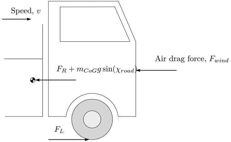
**Figure 7.3** Longitudinal forces acting on a vehicle.
