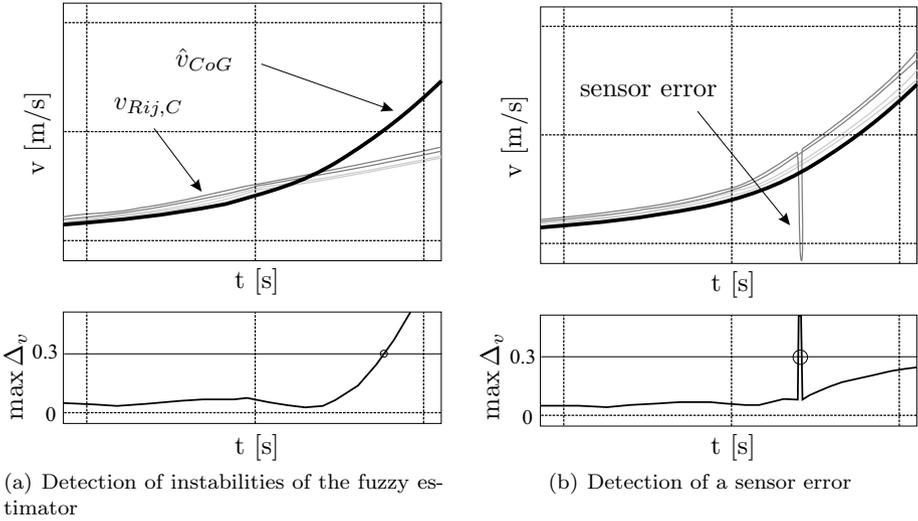
**Figure 9.9** Detection of errors using  $\max \Delta_v$
