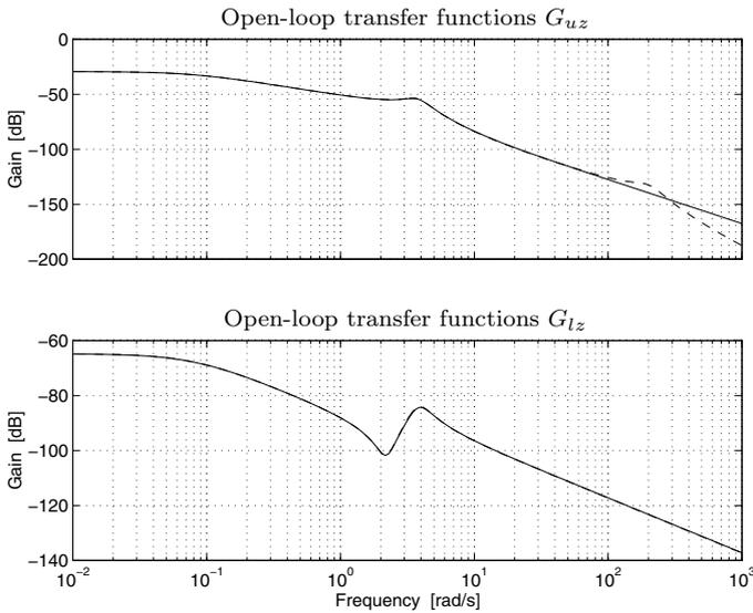
**Figure 7.39** Transfer functions from control signal,  $u$ , and load,  $l$ , to performance output,  $z$ . The Drive-shaft model is shown in solid and the Clutch and drive-shaft model is shown in dashed. The modeled clutch gives a second resonance peak and a steeper roll-off rate.
