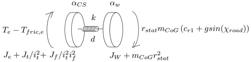
**Figure 7.9** The Drive-shaft model consists of a lumped engine and transmission inertia connected to the wheel inertia by a damped torsional flexibility.
