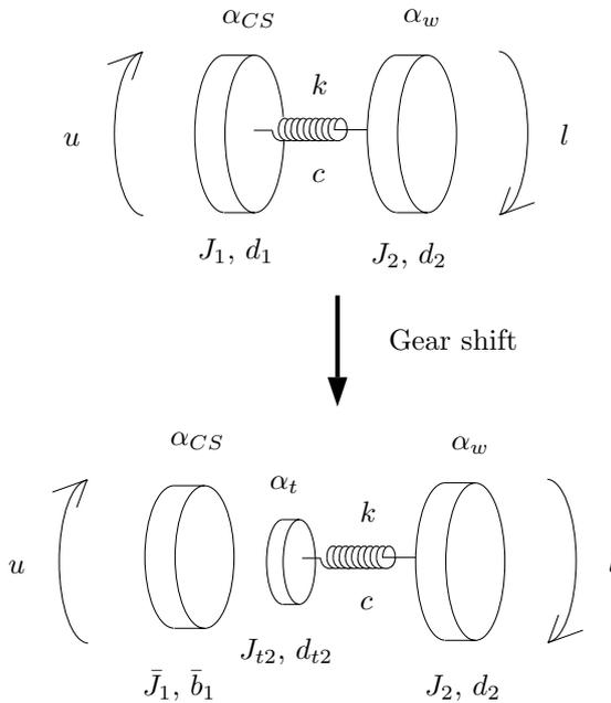
**Figure 7.24** Description of how the driveline model changes after engagement of neutral gear. The first model is the Drive-shaft model, which is then separated into two sub-models when neutral gear is engaged. The left part consists of the engine and one part of the transmission. The right part of the model consists of the rest of the transmission and the drive shaft out to the wheels, called the Decoupled model.
