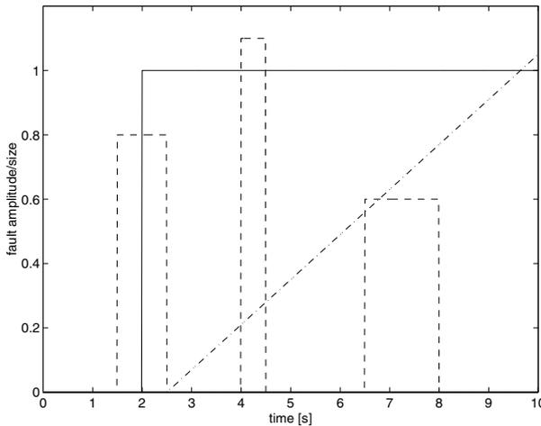
**Figure 6.4** Different types of fault time-variant behavior.
