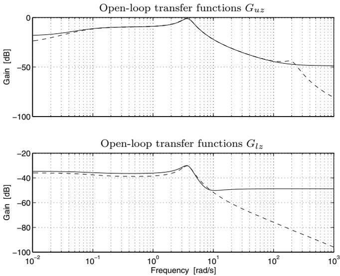
**Figure 7.53** Transfer functions from control signal,  $u$ , and load,  $l$ , to transmission torque,  $z$ . The Drive-shaft model is shown in solid and the Clutch and drive-shaft model is shown in dashed lines. The modeled clutch adds a second resonance peak and a steeper roll-off rate.
