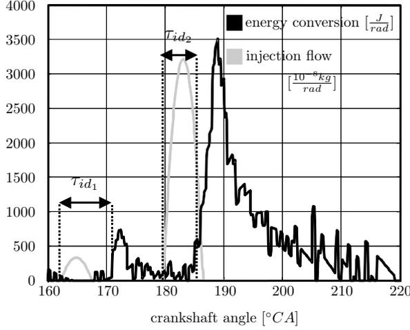
**Figure 4.9** Measured energy conversion and inflammation delay time
