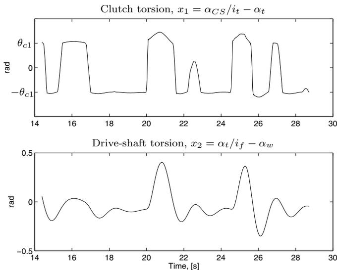
**Figure 7.19** Clutch torsion (top figure) and drive-shaft torsion (bottom figure) resulting from parameter estimation of the **Nonlinear clutch and drive-shaft model** with sensor filtering, on data with gear 1. The true values of these torsions are not known, but the plots show that they have realistic values.
