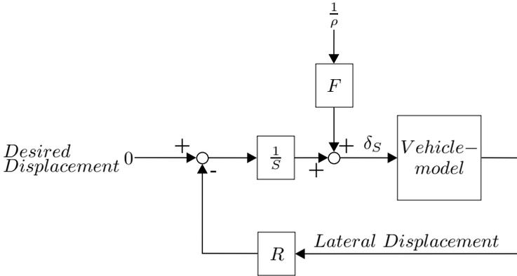
**Figure 11.30** Simplified block diagram of the lateral control with feed forward
