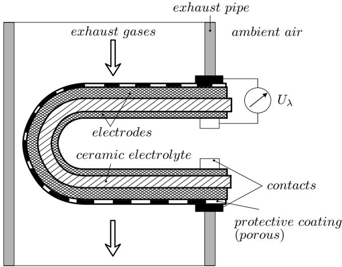
Figure 5.5 Zirconium dioxide sensor
