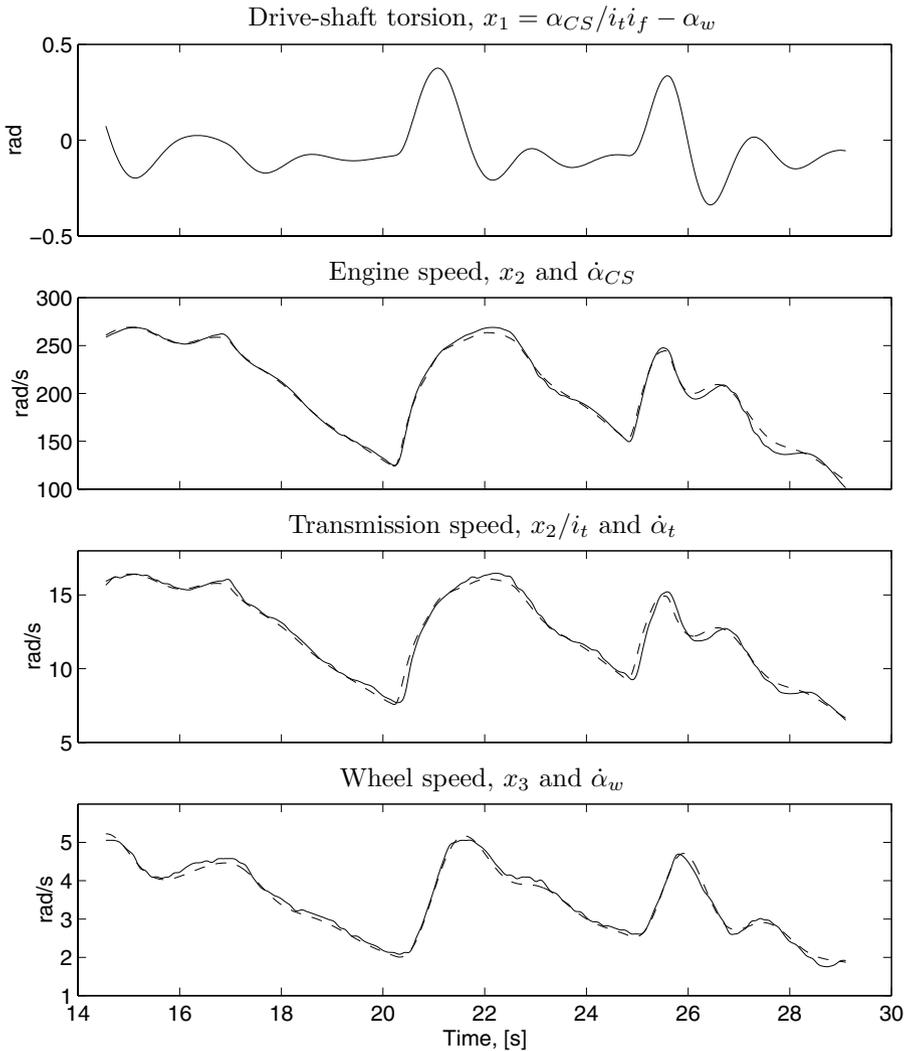
**Figure 7.10** The parameters of the Drive-shaft model estimated on data with step inputs in accelerator position using gear 1. The top figure shows the estimated drive-shaft torsion, and the bottom figures show the model outputs ( $x_2$ ,  $x_3$ ) in dashed lines, together with the measured driveline speeds in solid. The plots are typical examples of that a major part of the dynamics is captured by a linear model with a drive-shaft flexibility.
