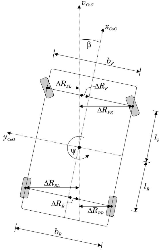
Figure 8.8 Differential curve radii of the individual wheels
