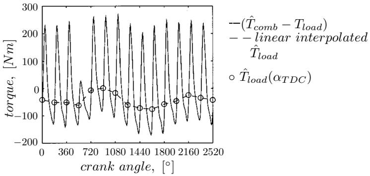
**Figure 6.25** Estimated combustion torque difference by Kalman filter
