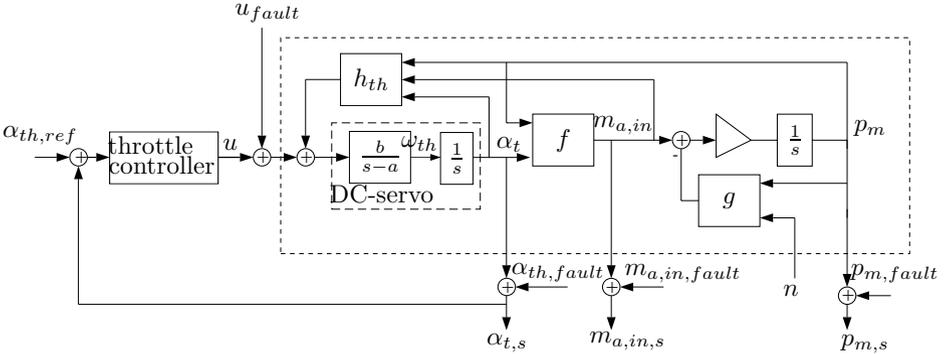
**Figure 6.11** The model of the air intake system including the throttle controller and monitored faults.
