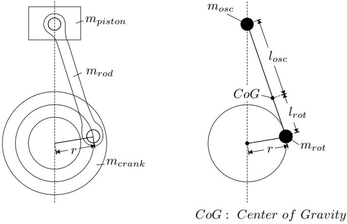
**Figure 6.21** Two-mass model for oscillating and rotating masses.
