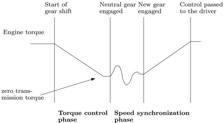
**Figure 7.26** Engine torque during the different phases in automatic gear shifting by engine control. The engine torque is controlled to a state where the transmission transfers zero torque, whereafter neutral gear is engaged without using the clutch. After the speed synchronization phase, the new gear is engaged, and control is transferred back to the driver.
