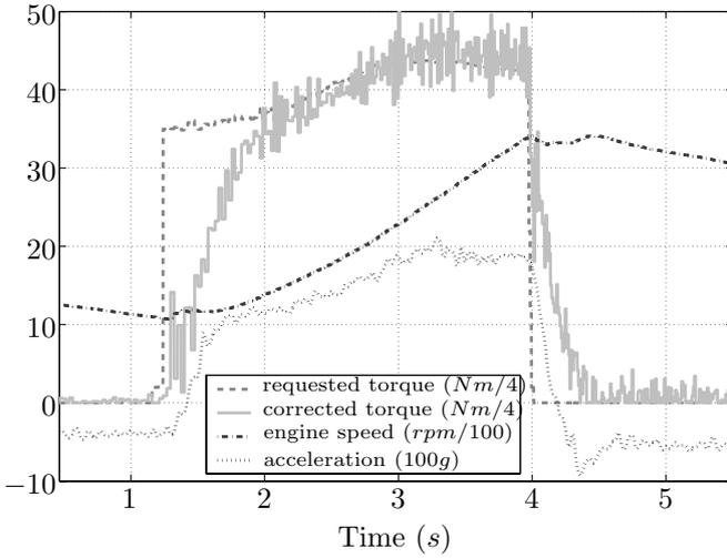
(a) Torque, Engine Speed and Acceleration
