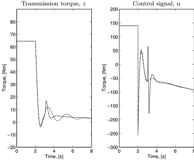
**Figure 7.63** Same simulation case as in Figure 7.61, but with a load disturbance at  $t=3$  s. Feedback from the wheel-speed sensor is shown in solid lines, and feedback from the engine-speed sensor is shown in dashed lines. The conclusion is that the load disturbance is better attenuated when using feedback from the wheel-speed sensor.
