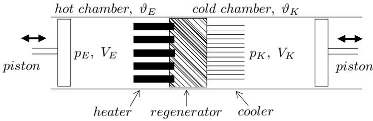
**Figure 2.19** Mechanical representation of the Stirling engine
