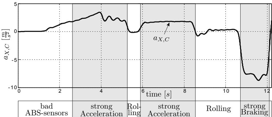
**Figure 9.10** Corrected longitudinal acceleration  $a_{x,C}$  categorizing the driving situation
