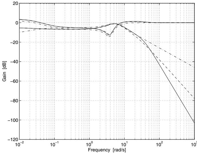
**Figure 7.59** Sensitivity function  $S$  and complementary sensitivity function  $T$ . The dash-dotted lines correspond to the case with all states known. When only one velocity is measured, the solid lines correspond to  $\dot{\alpha}_w$ -feedback, and the dashed lines correspond to  $\dot{\alpha}_{CS}$ -feedback.
