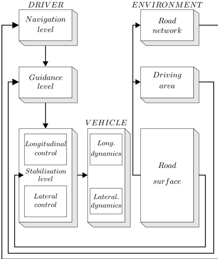
**Figure 11.7** The three level hierarchy of vehicle control
