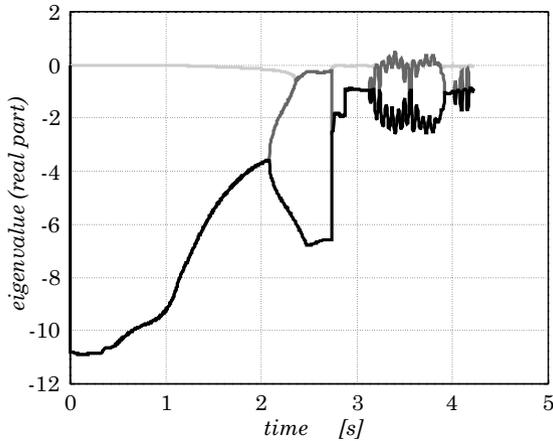
**Figure 8.31** Real part of the eigenvalues during braking manoeuvre in a curve
