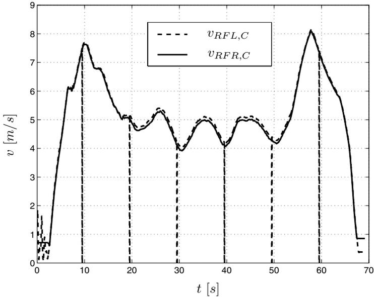
Figure 9.21 Artificially induced errors of ABS-sensor (front left)
