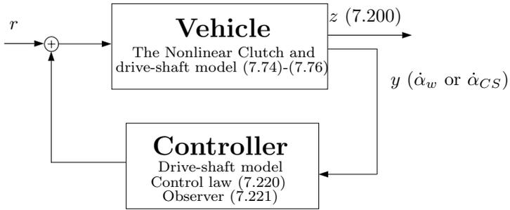
**Figure 7.60** Simulation configuration. As a step for demonstrating feasibility for real implementation, the Nonlinear clutch and drive-shaft model is simulated with the controller based on the Drive-shaft model.
