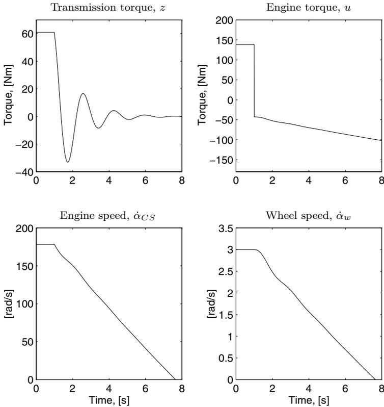
**Figure 7.55** The Drive-shaft model controlled with the gear-shift condition (7.207). At  $t=1$  s, a gear shift is commanded. The speed dependent realizable control signal drives the transmission torque to zero. Undamped oscillations in the transmission torque increase the time needed to fulfill the goal of controlling the transmission torque to zero.
