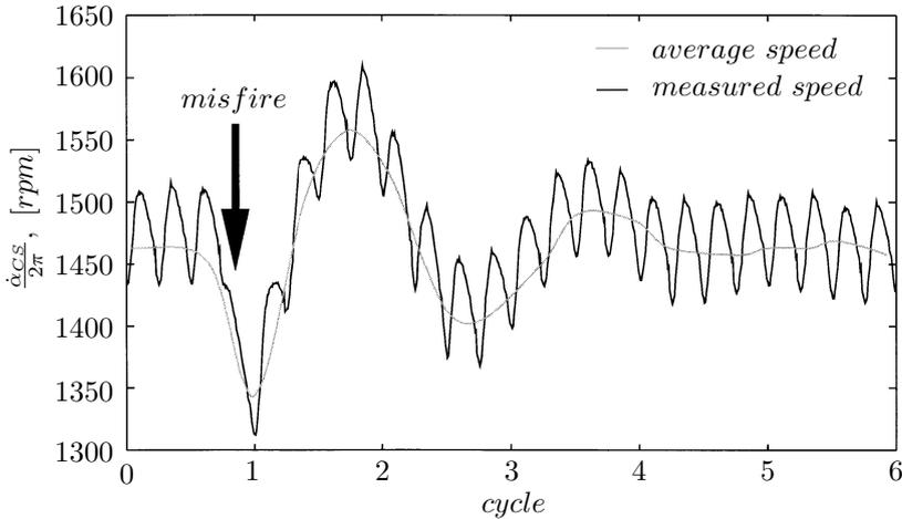
**Figure 6.24** Measured angular speed signal with single misfire
