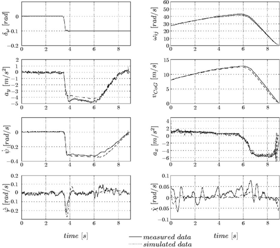
**Figure 8.33** Model validation: step change in steering angle
