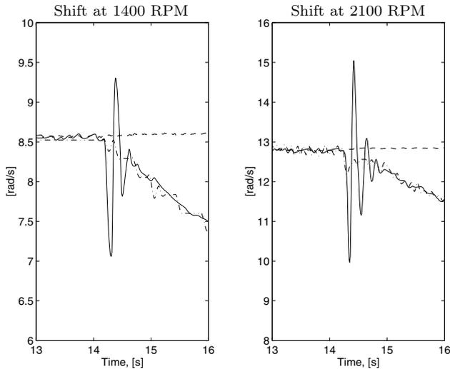
**Figure 7.28** Engagement of neutral gear commanded at 14 s, with stationary driveline at 1400 RPM and 2100 RPM on a flat road with gear 1. The engine speed (dashed) and wheel speed (dash-dotted) are scaled to transmission speed (solid) with the conversion ratio of the driveline. After a short delay time, neutral gear is engaged, causing the driveline speeds to oscillate. The amplitude of the oscillating transmission speed is higher the higher the stationary speed is.
