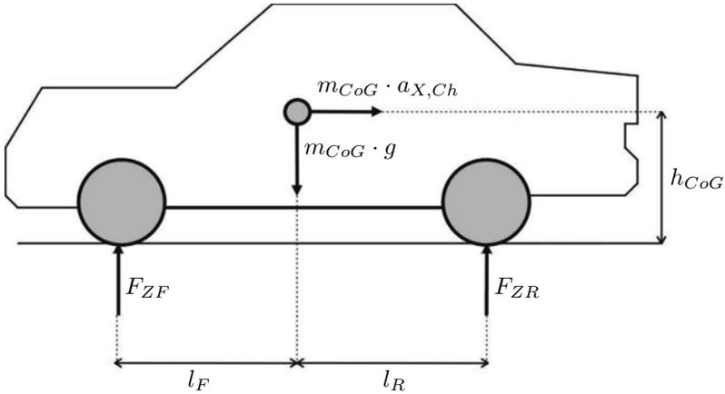
**Figure 9.33** Axle load shifting during acceleration
