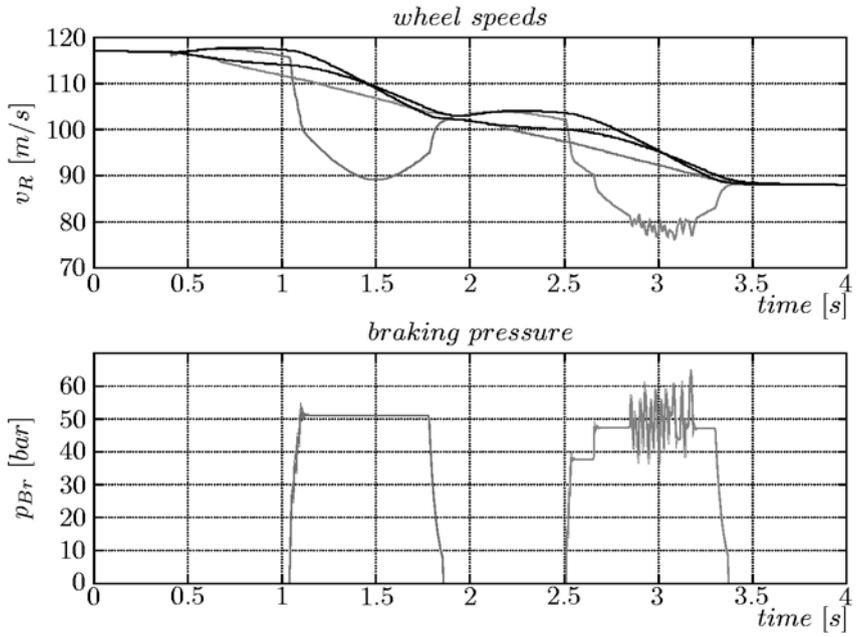
**Figure 10.14** Rotational equivalent velocities and stabilizing brake pressure
