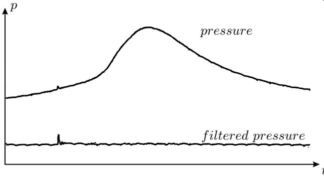
**Figure 5.38** Bandpass output signal for non-knocking combustion
