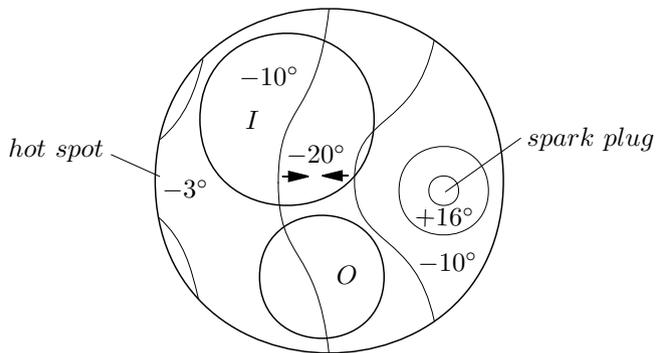
**Figure 5.32** Self-ignition with two colliding flame fronts
