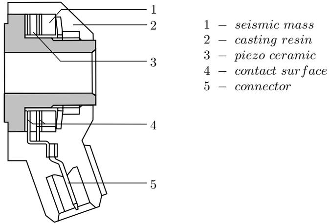
Figure 5.34 Mechanical knock sensor
