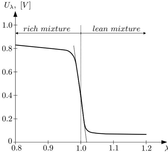
**Figure 5.6** Output voltage of zirconium dioxide sensor
