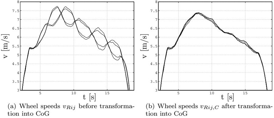
**Figure 9.2** Wheel speeds during a sinusoidal drive
