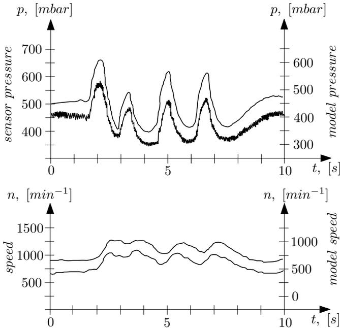
**Figure 5.26** Comparison of measured and calculated manifold pressure
