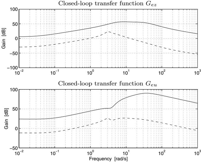
**Figure 7.58** Closed-loop transfer functions from measurement noise,  $e$ , to performance output,  $z$ , and control signal,  $u$ . Feedback from  $\dot{\alpha}_w$  is shown in solid and feedback from  $\dot{\alpha}_{CS}$  is shown in dashed. The difference between the two feedback principles are described by the dynamic output ratio. The effect increases with lower gears.
