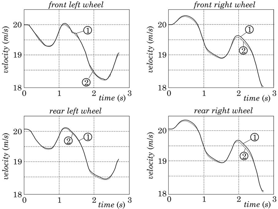
**Figure 8.10** Comparison of the two methods for the derivation of the wheel ground contact point velocities
