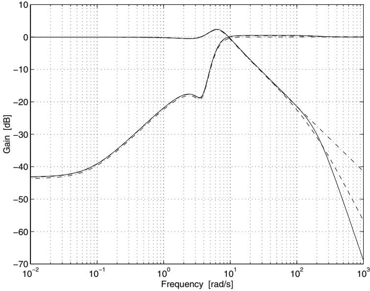
**Figure 7.45** Sensitivity function  $S$  and complementary sensitivity function  $T$ . The dash-dotted lines correspond to the case with all states known. When only one velocity is measured, the solid lines correspond to  $\hat{\alpha}_w$ -feedback, and the dashed lines correspond to  $\hat{\alpha}_{CS}$ -feedback.
