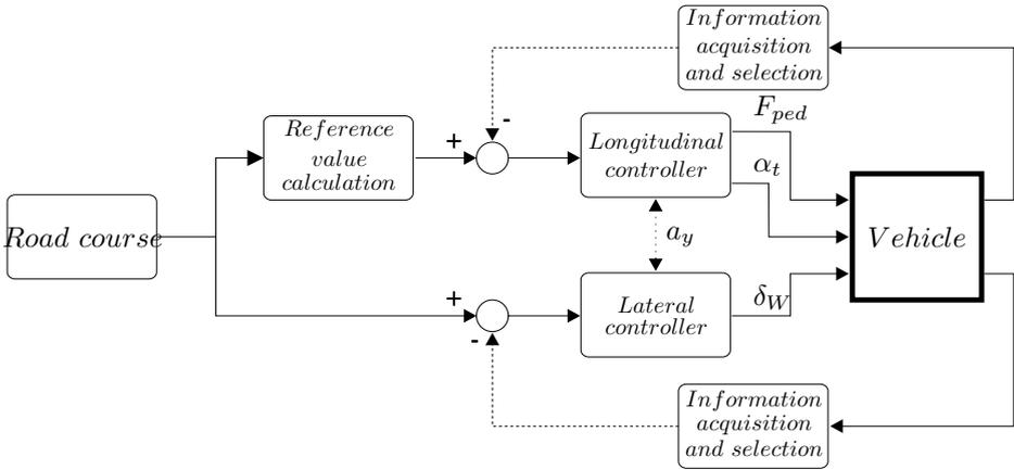
Figure 11.19 Controller structure
