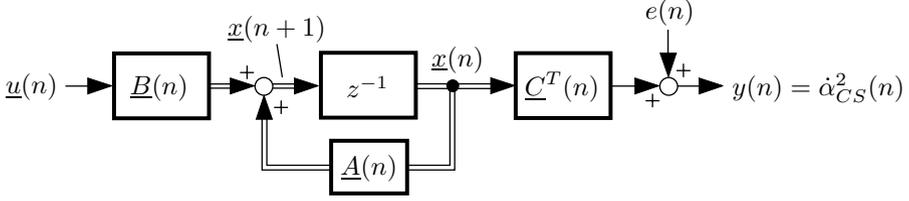
$$\begin{aligned}\underline{x}(n+1) &= \underline{A}(n)\underline{x}(n) + \underline{B}(n)\underline{u}(n) \\ \underline{y}(n) &= \underline{C}(n)\underline{x}(n) + \underline{e}(n)\end{aligned}$$
