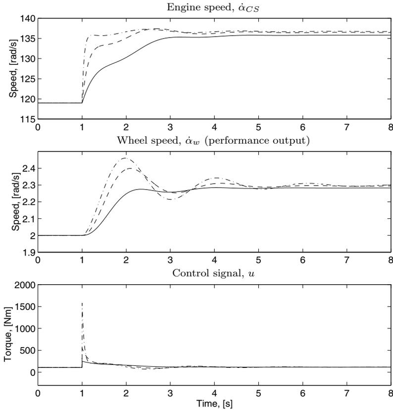
**Figure 7.37** Response of step in accelerator position at  $t=1$  s, with RQV control (7.115) controlling the Drive-shaft model. Controller gains  $K_p=8$ ,  $K_p=25$ , and  $K_p=85$  are shown in solid, dashed, and dash-dotted lines respectively. Increased gain results in a well damped engine speed and an oscillating wheel speed.
