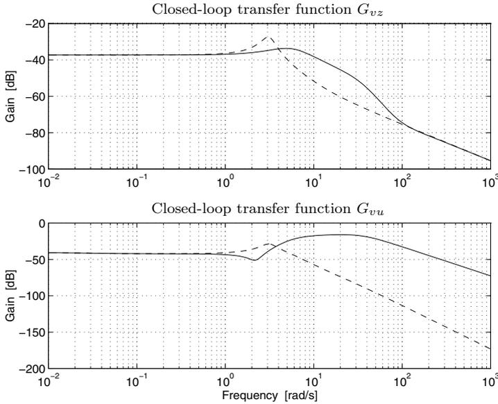
**Figure 7.57** Closed-loop transfer functions from load disturbance,  $v$ , to performance output,  $z$ , and to control signal,  $u$ . Feedback from  $\dot{\alpha}_w$  is shown in solid and feedback from  $\dot{\alpha}_{CS}$  is shown in dashed lines. With  $\dot{\alpha}_{CS}$ -feedback the transfer functions have a resonance peak, resulting from the open-loop zeros.
