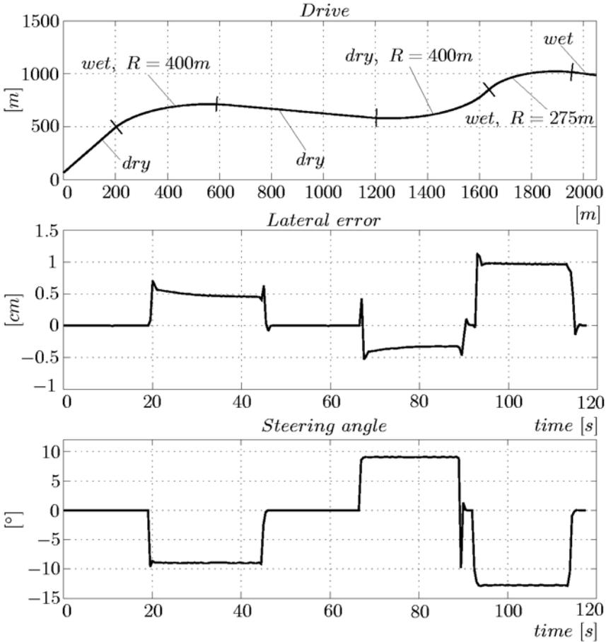
**Figure 11.32** Simulation results for the lateral controller
