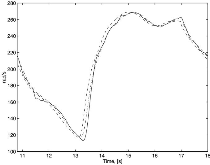
**Figure 7.15** Enlargement of part of Figure 7.14. Measured transmission speed (solid), output from the Drive-shaft model without sensor filtering (dashed), and output from the Drive-shaft model with sensor filtering (dash-dotted). The parameters are estimated based on experiments with gear 1.
