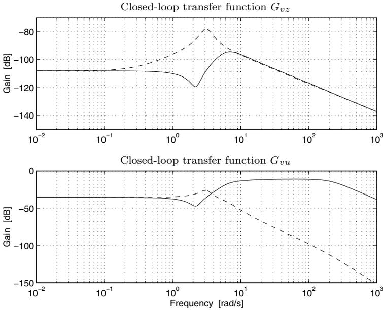
**Figure 7.42** Closed-loop transfer functions from load disturbance,  $v$ , to performance output,  $z$ , and to control signal,  $u$ . Feedback from  $\dot{\alpha}_w$  is shown in solid and feedback from  $\dot{\alpha}_{CS}$  is shown in dashed lines. With  $\dot{\alpha}_{CS}$ -feedback the transfer functions have a resonance peak, resulting from the open-loop zeros.
