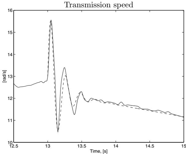
**Figure 7.25** Measured oscillations after a gear shift at 13.0 s in solid line. The outputs of the Decoupled model are fitted to data, shown in dashed line. The Decoupled model is able to capture the main resonance in the oscillating transmission speed after the gear shift.
