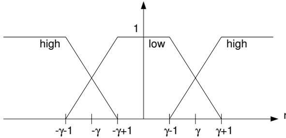
**Figure 6.14** The fuzzy sets used in the fuzzy thresholding.
