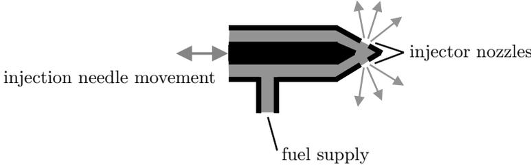
**Figure 4.4** Schematic structure of an injector.
