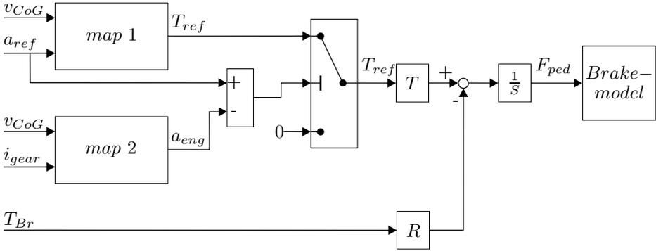
**Figure 11.29** Simplified block diagram of the brake controller
