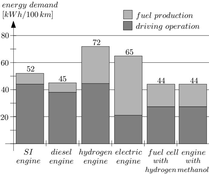
**Figure 2.24** Energy demand of different engine concepts [74]
