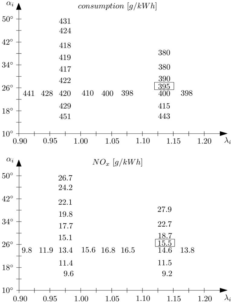
**Figure 3.21** Fuel consumption and  $NO_x$  emissions over ignition angle  $\alpha_i$  and air-fuel ratio  $\lambda$  at an operating point  $i$  with  $L_{NO_x} = 3$ .
