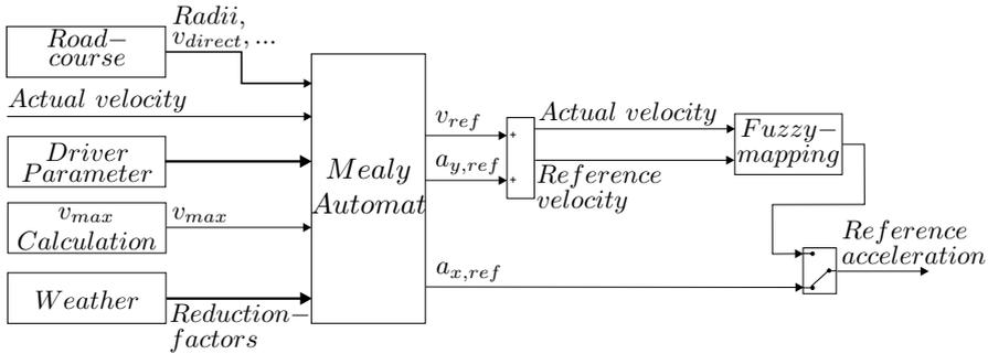
Figure 11.17 Structure of reference value calculation
