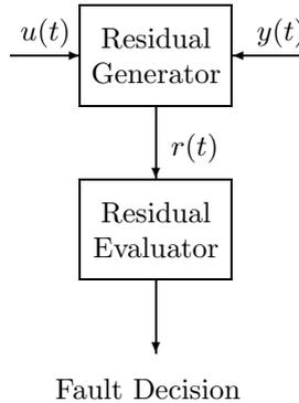
**Figure 6.5** Internal structure of a diagnosis system.
