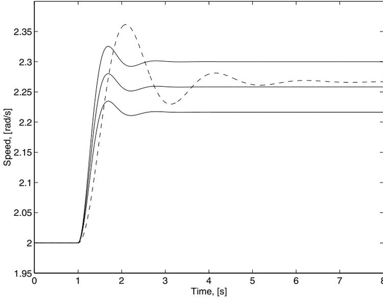
**Figure 7.41** Wheel-speed response of step in accelerator position at  $t=1$  s. The Drive-shaft model is controlled with the RQV controller (7.115) in dashed line, and the speed controller with stationary error (7.140) with  $\beta = 0, 0.5, 1$  in solid lines. The speed controller achieves the same stationary level as the RQV controller by tuning  $\beta$ .
