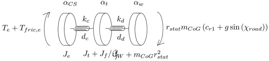
**Figure 7.16** The Clutch and drive-shaft model: Linear clutch and drive-shaft torsional flexibility.
