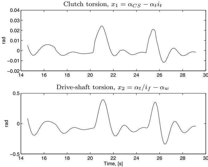
**Figure 7.17** Clutch torsion (top figure) and drive-shaft torsion (bottom figure) resulting from parameter estimation of the Clutch and drive-shaft model with sensor filtering, on data with gear 1. The true values of these torsions are not known, but the plots show that the drive-shaft torsion has realistic values.
