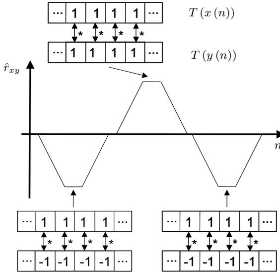
**Figure 10.7** Sequence of tri-state correlation coefficients of a single ABS-cycle pattern
