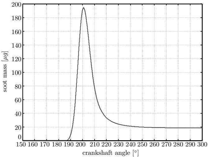
**Figure 4.14** Soot mass as difference between accrueement and oxidation over crankshaft angle
