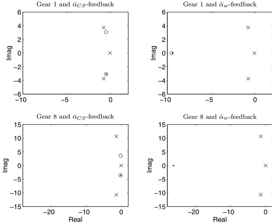
**Figure 7.31** Root locus with respect to a P-controller gain, for gear 1 (top figures) and gear 8 (bottom figures), with sensor on  $\dot{\alpha}_{CS}$  (left figures), or  $\dot{\alpha}_w$  (right figures). The cross represent the open-loop poles, while the rings represent the open-loop zeros. The system goes unstable when the  $\dot{\alpha}_w$ -gain is increased, but is stable for all  $\dot{\alpha}_{CS}$ -gains.
