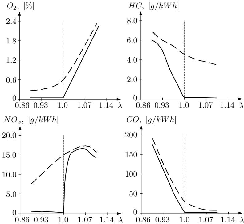
**Figure 5.1** Measurement of exhaust gases: oxygen  $O_2$ , hydrocarbon  $HC$ , nitrogen oxide  $NO_x$  and carbon monoxide  $CO$ . The concentration before the catalytic converter are indicated by dotted and the concentrations after the catalytic converter by straight lines.
