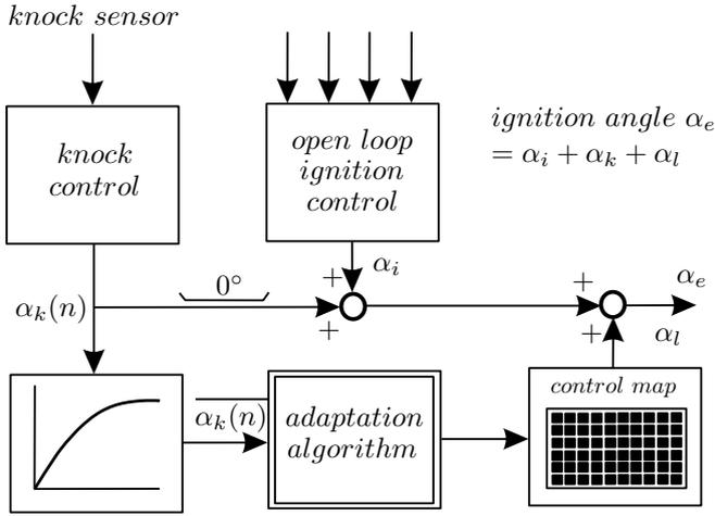
**Figure 5.41** Knock control with feed-forward adaptive ignition angle map
