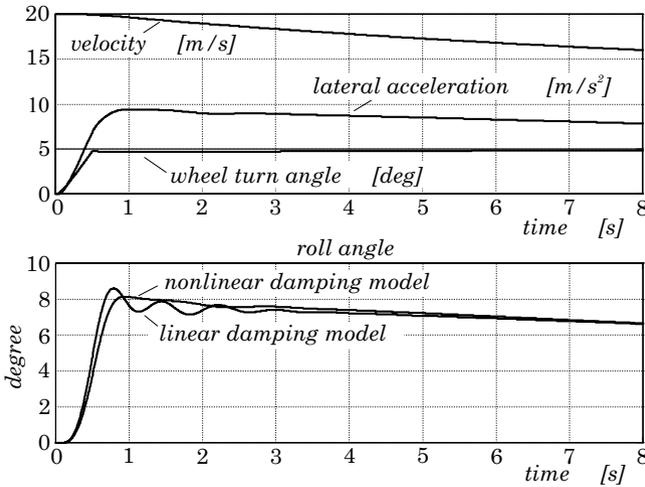
**Figure 8.29** Roll angle from linear and nonlinear suspension models
