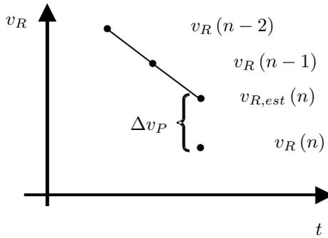
Figure 10.5 Sketch of extrapolated wheel speed signal
