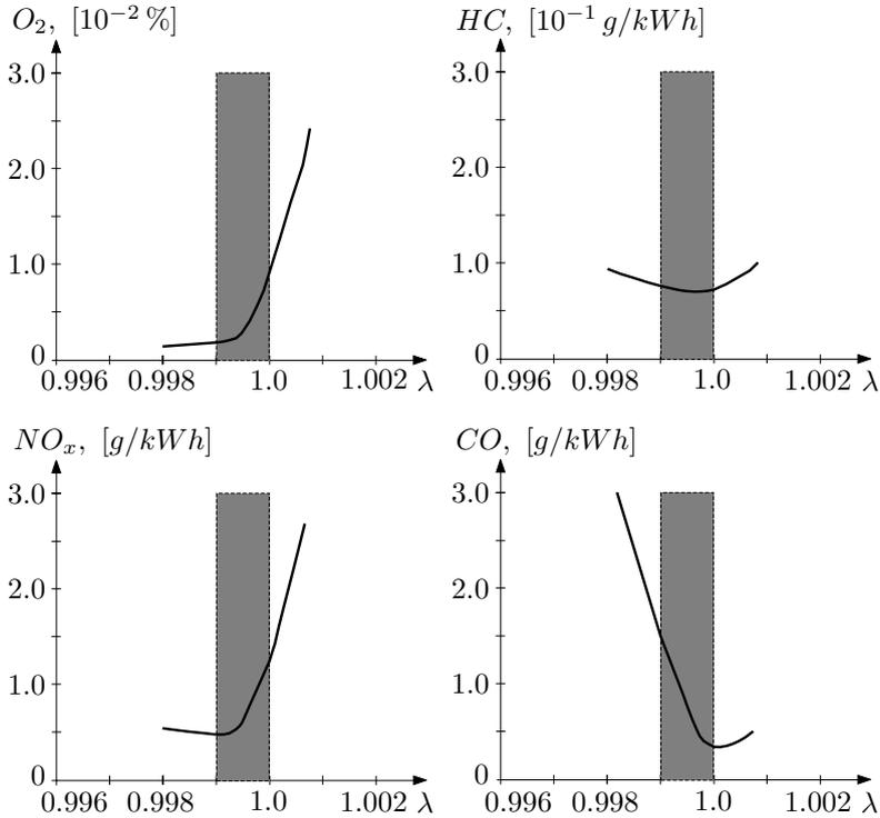
**Figure 5.2** Emission rates of an engine after the catalytic converter at a static operating point (engine speed 1800 rpm and torque  $T = 65 Nm$ ). Average lambda (500 cycles) should be within the indicated window.
