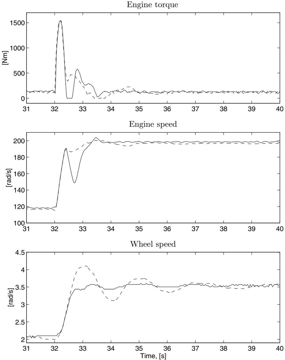
**Figure 7.50** Speed step at  $t=32$  s with active damping and engine-speed feedback (solid) compared to traditional RQV control with  $K_p=50$  (dashed). Experiments are performed on a flat road. After 32.5 s, the control signals differ depending on control scheme. With speed control, the engine inertia works in the opposite direction of the oscillations, which are significantly reduced.
