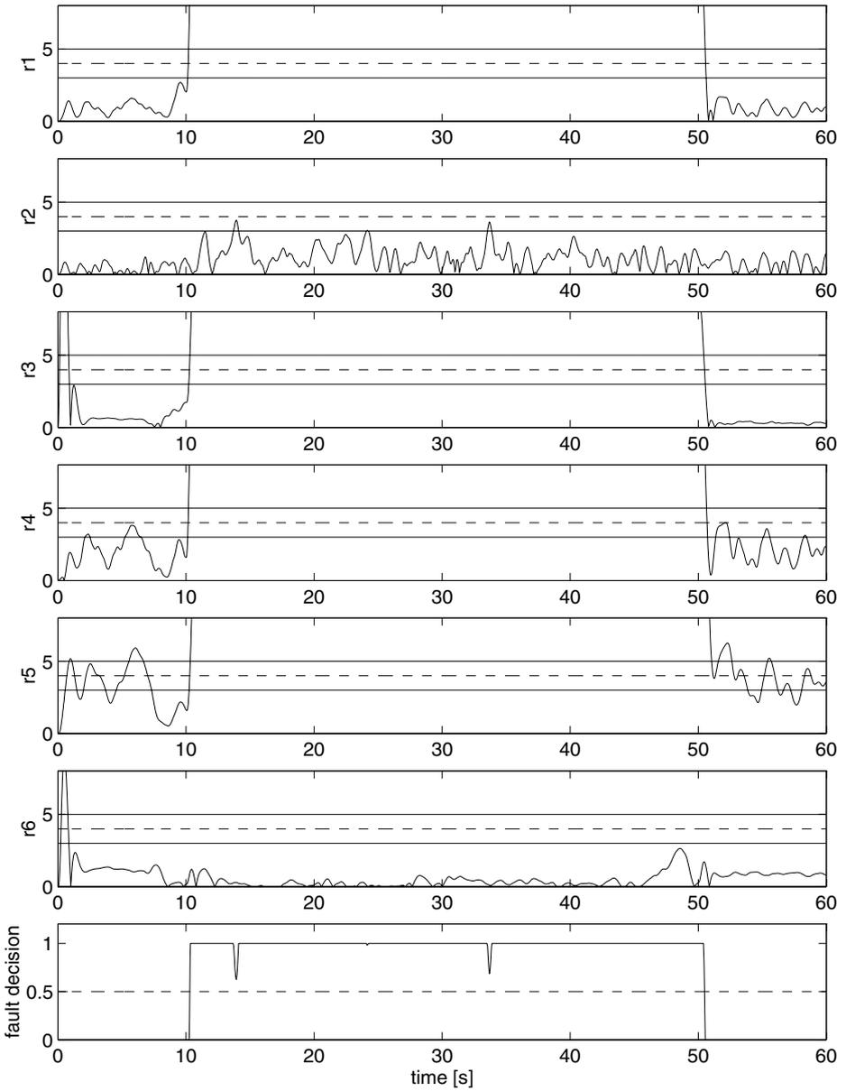
**Figure 6.18** The residuals for 10% throttle sensor fault.
