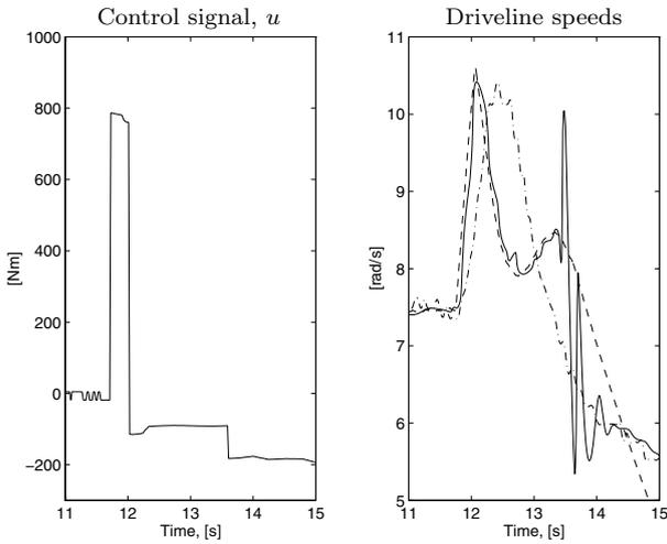
**Figure 7.23** Same field trial as in Figure 7.22, but with engaged neutral gear at 13.2 s. Engine speed (dashed) and wheel speed (dash-dotted) are scaled to transmission speed (solid) in the right figure. After the gear shift the transmission speed oscillates.
