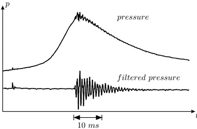
**Figure 5.39** Bandpass output signal for knocking combustion
