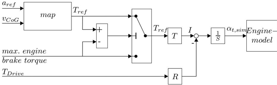
**Figure 11.28** Block diagram of the drive controller
