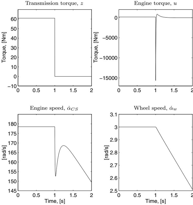
**Figure 7.54** Unconstrained active damping of the Drive-shaft model. At  $t=1$  s, a gear shift is commanded and the control law (7.202) calculates the engine torque such that the transmission torque is driven to zero instantaneously. The oscillations in the transmission torque are damped with an unrealizable large control signal. The wheel speed decreases linearly.
