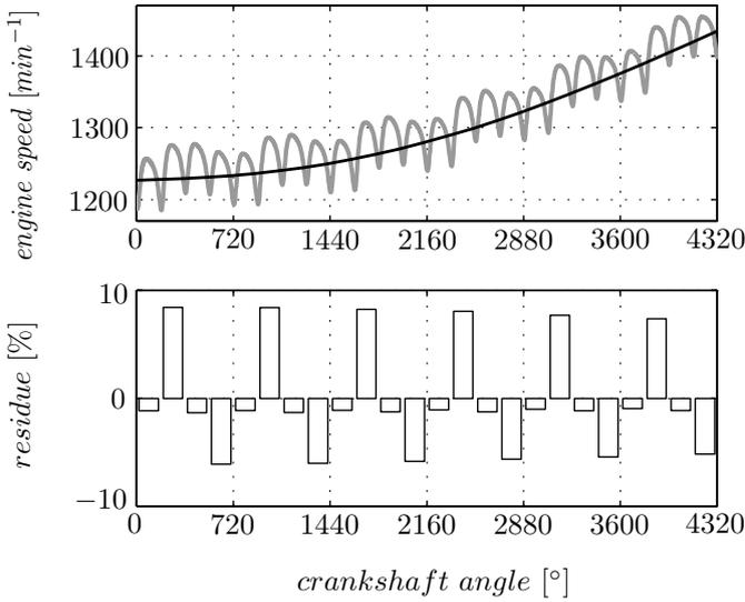
Figure 5.48 Compensated residues at 4-cylinder engine during transient
