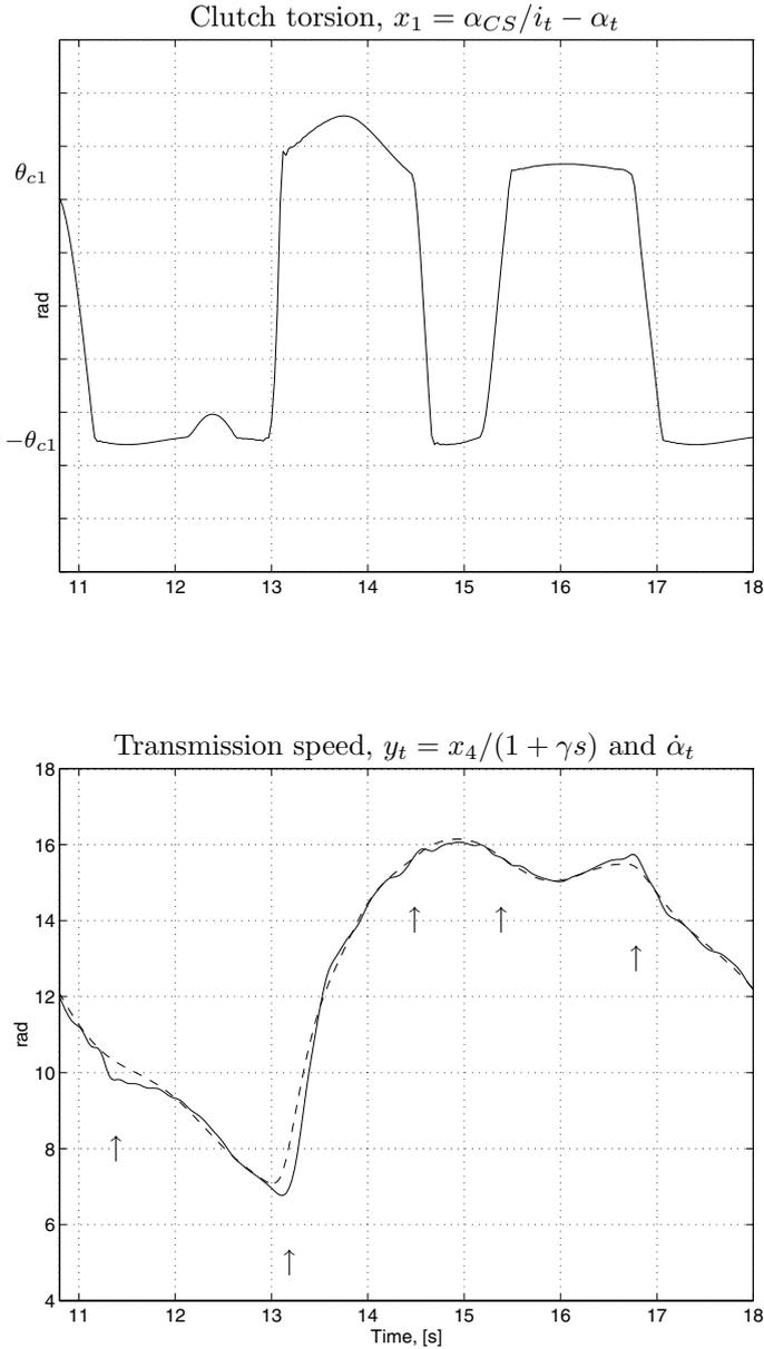
**Figure 7.20** Clutch torsion (top figure) and measured and estimated transmission speeds (bottom figure) from the Nonlinear clutch and drive-shaft model with sensor dynamics with gear 1. The result is that the main differences between model (dashed) and experiments (solid) occur when the clutch torsion passes the area with the low stiffness ( $|\theta| < \theta_{c1}$ ) in the static clutch nonlinearity.
