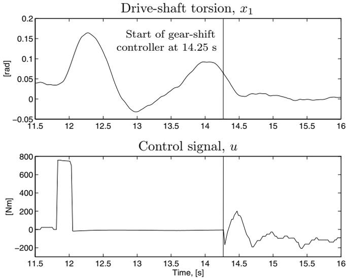
**Figure 7.70** Control signal and drive-shaft torsion during field trials with start of the gear-shift controller at 14.25 s. The controller controls the drive-shaft torsion to zero with damped resonances despite initial driveline oscillations.
