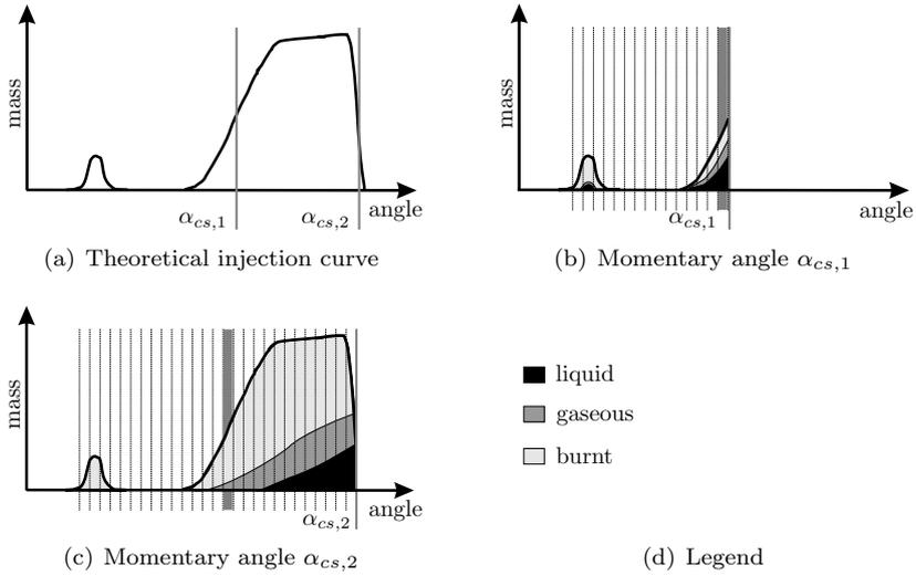
**Figure 4.7** Schematic sequence of the evaporation process.
