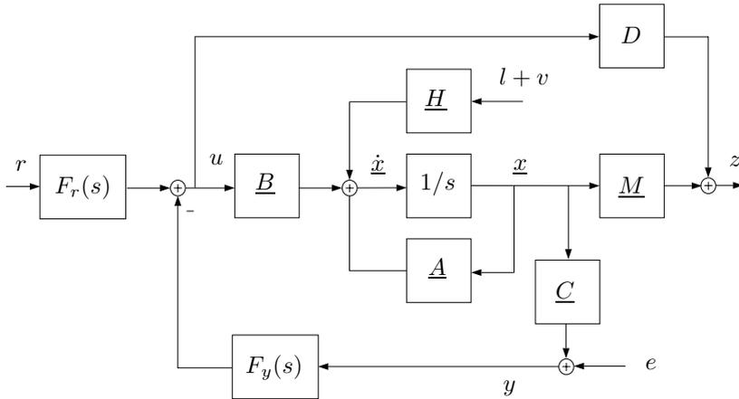
Figure 7.30 Plant and controllers  $F_r$  and  $F_y$ .
