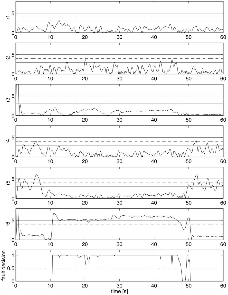
**Figure 6.17** The residuals for 20% throttle actuator fault.
