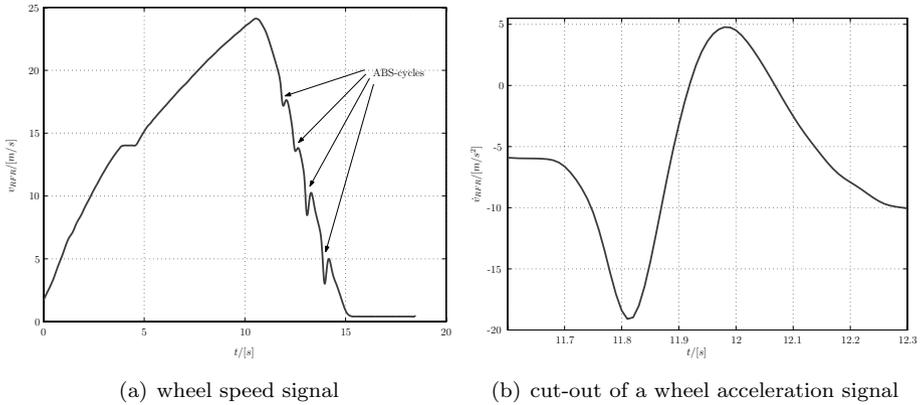
Figure 10.4 Pattern of an ABS-cycle
