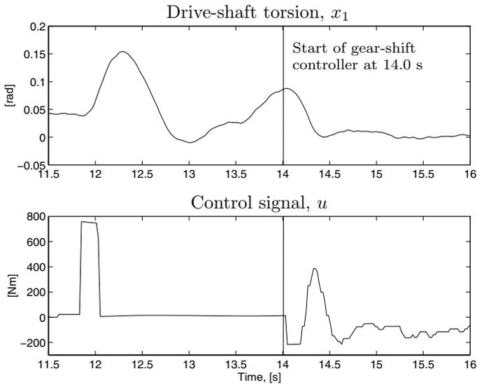
**Figure 7.69** Control signal and drive-shaft torsion during field trials with start of the gear-shift controller at 14.0 s. The controller controls the drive-shaft torsion to zero with damped resonances despite initial driveline oscillations.
