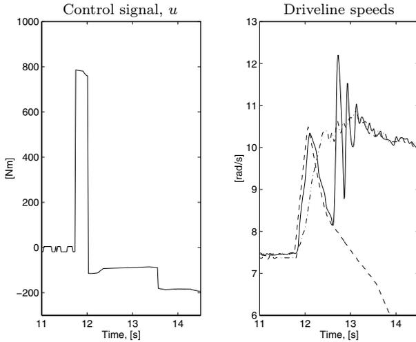
**Figure 7.22** Engaged neutral gear without torque control at 12.5 s in a trial with oscillating driveline as a result of a provoking engine torque pulse at 11.7 s in the left figure. Engine speed (dashed) and wheel speed (dash-dotted) are scaled to transmission speed (solid) in the right figure. After the gear shift the transmission speed oscillates.
