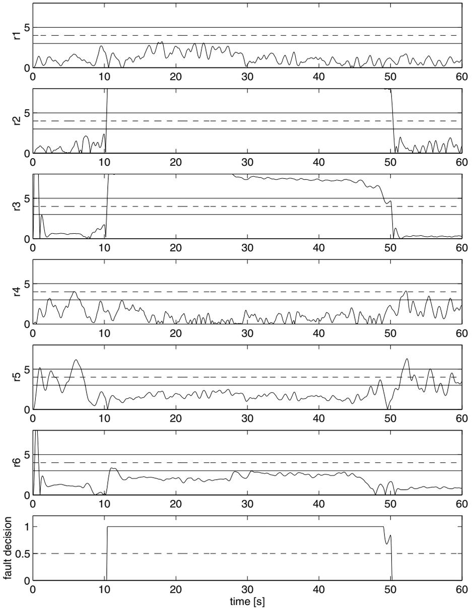
**Figure 6.20** The residuals for 10% manifold pressure sensor fault.
