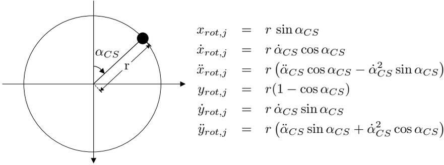
**Figure 6.22** Rotational Motion at the crankshaft
