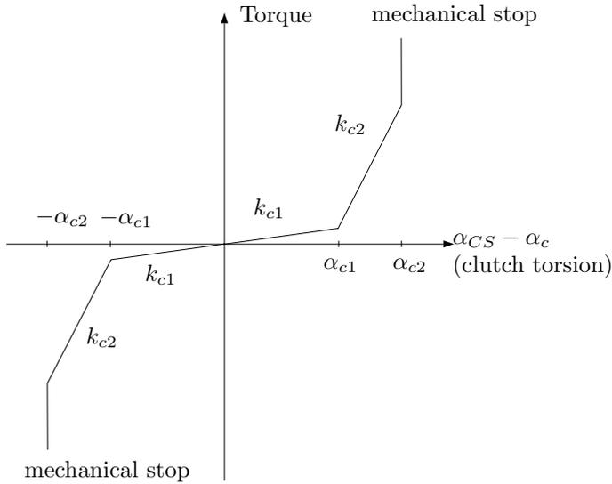
Figure 7.18 Nonlinear clutch characteristics.
