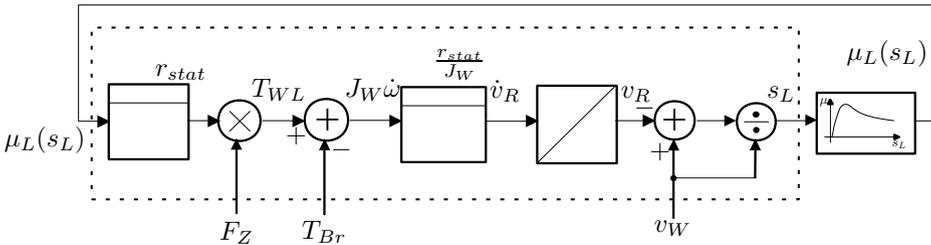
Figure 10.2 Block diagram of torque balance at wheel base
