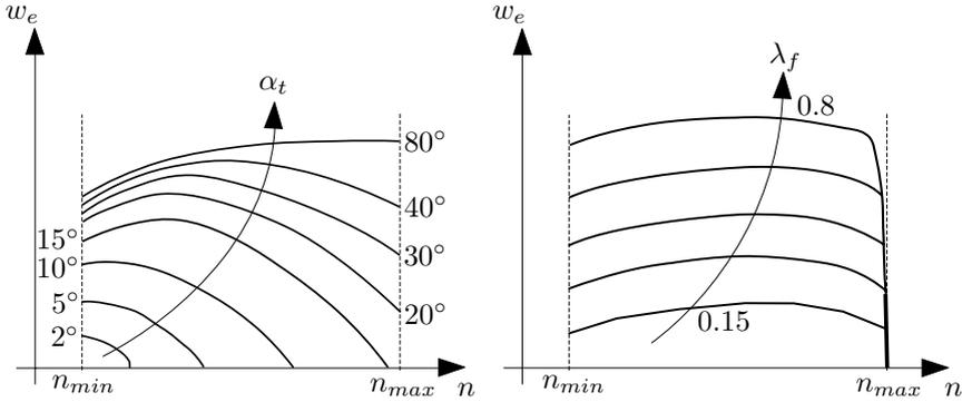
**Figure 3.5** Effective work  $w_e$  over engine speed for SI engines (left figure) depending on the throttle angle  $\alpha_t$  and Diesel engines (right figure) depending on relative fuel supply  $\lambda_f$ .
