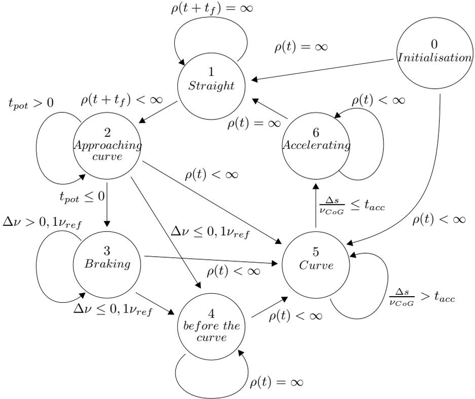
Figure 11.18 State graph of the finite automat
