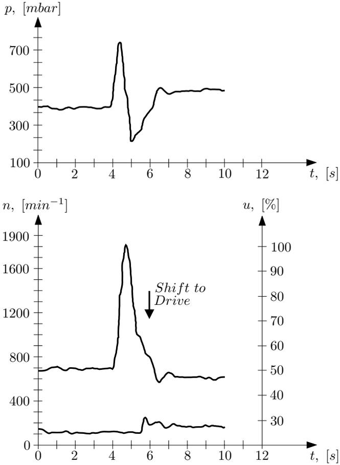
**Figure 5.31** Disturbance input from driver and simultaneous gear shift to Drive position
