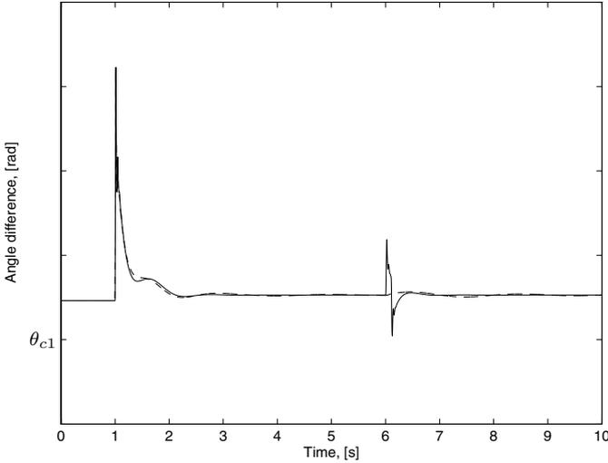
**Figure 7.49** Clutch-angle difference corresponding to Figure 7.47. The influence from the clutch nonlinearity can be neglected, because the area with low stiffness ( $\alpha_c < \alpha_{c1}$ ) is never entered.
