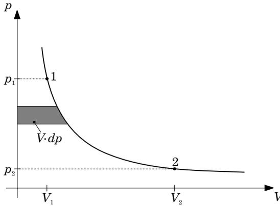
**Figure 2.2** Mechanical work due to pressure change
