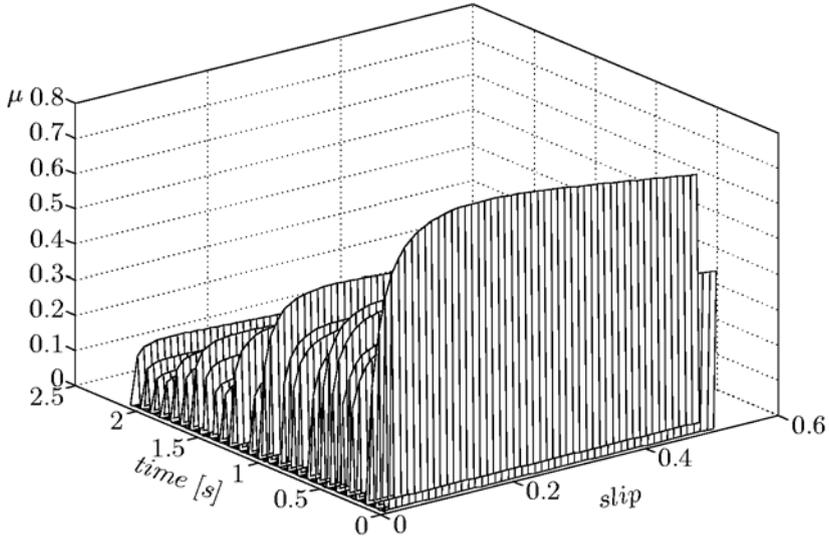
**Figure 9.26** Estimated friction characteristic for the front left wheel (wet grass)
