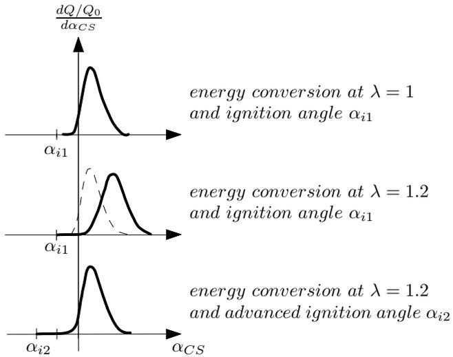
**Figure 3.11** Normalized energy conversion caused by combustion for different air-fuel ratios  $\lambda$ .
