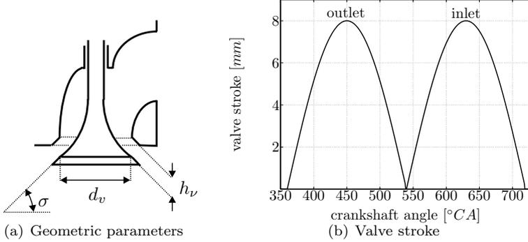
**Figure 4.2** Cross sectional area at the valves.
