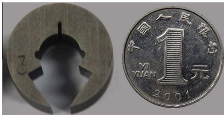
Fig. 1b. The real picture of a CIET specimen.
