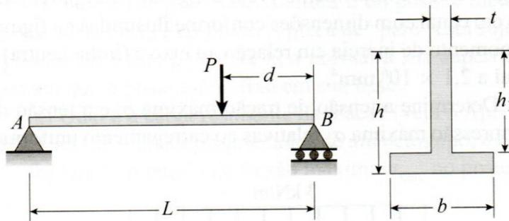
$$\sigma_{\max} = \frac{M_{\max}}{I} c_2 \quad \sigma_c = \frac{M_{\max}}{I} c_1$$
