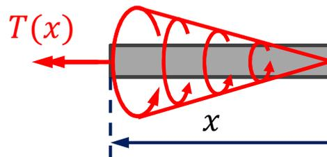
$$T(x) = \int_0^x t(x) dx = \int_0^x \frac{t_A x}{L} dx = \frac{t_A x^2}{2L}$$
