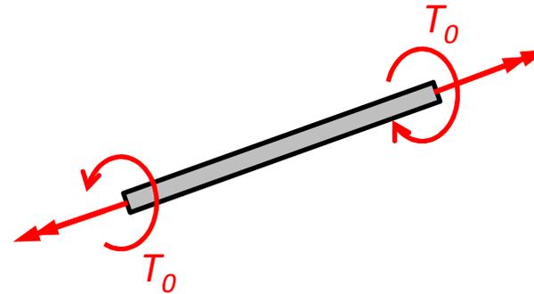
$$T_0 = P \times 2L = 25 \text{ lbf} \times 2 \times 9 \text{ in} = 450 \text{ lbf} \cdot \text{in}$$
