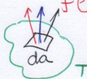
The diagram shows a small square area labeled 'da' inside a larger irregular shape representing a body at temperature 'T'. Three arrows point upwards from the square, representing the emission of radiation.
