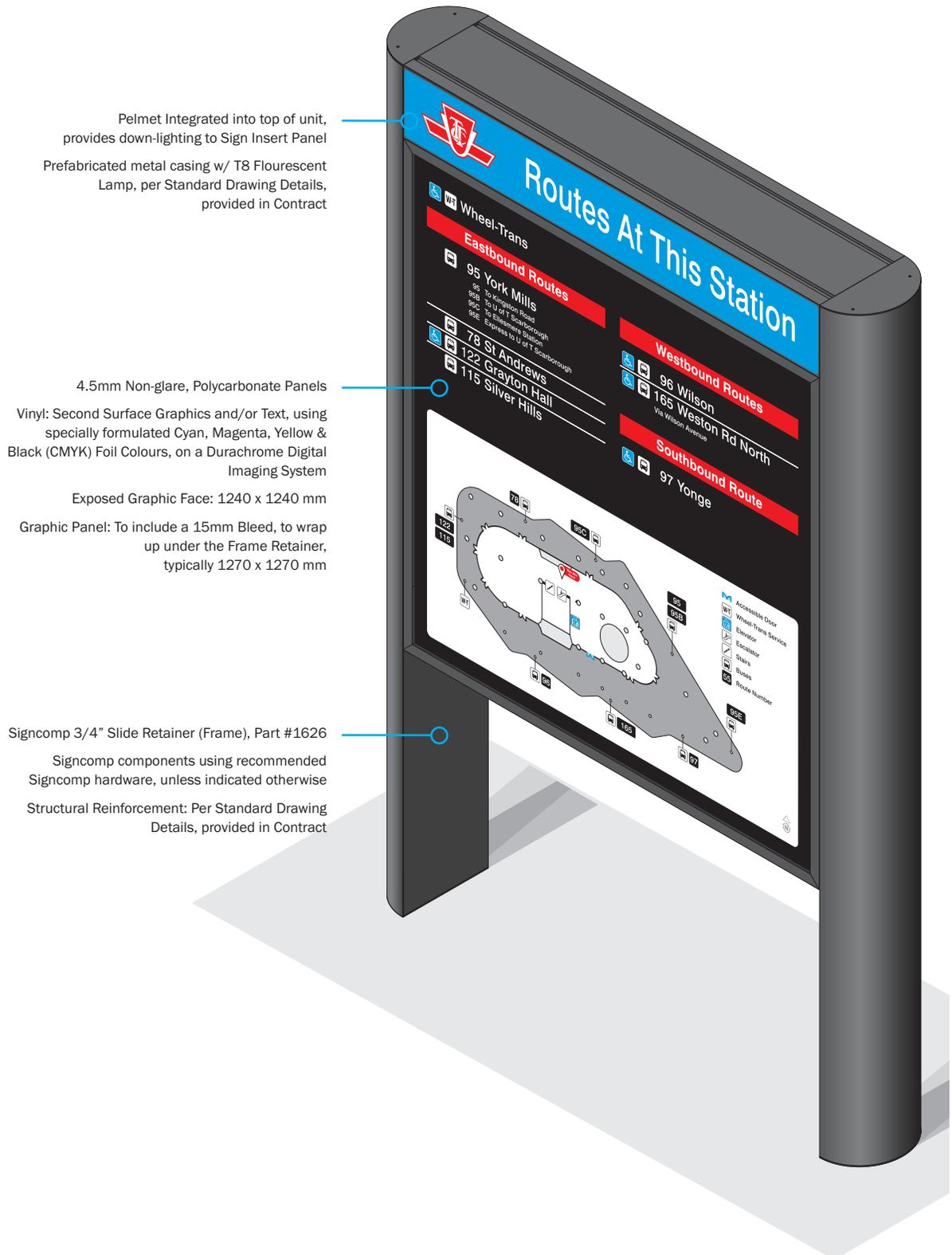
Pelmet Integrated into top of unit, provides down-lighting to Sign Insert Panel
