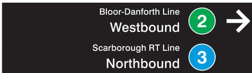
Sign messages should be ranged left or right according to the direction indicated by the arrow. Arrow should appear to *drag* the symbols and message.
